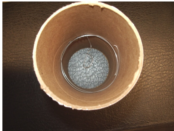
Fig. 7. Aluminum wire support in cardboard canister (7.63 cm diameter).
