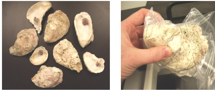
Fig 11. Oyster shells of various sizes and thicknesses (left) and an oyster phantom (right). The phantoms consisted of two oyster shells of similar thicknesses covering a plastic bag filled with water. The FIC was placed inside the phantom.
