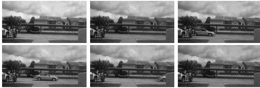
Fig. 45. Frame Seq. 2: outdoor variable lighting due to clouds. The light intensity changes by 70% between frames. Additional background movement due to shrub.
