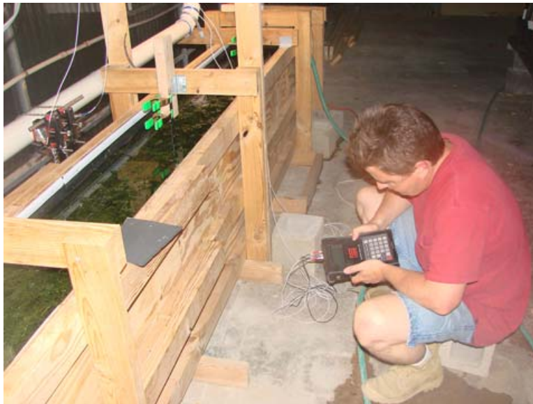
Fig. 3.5. Greenhouse channel showing staff gage setup. Note Panamatrix transit time meter clamped to recirculation pipeline
