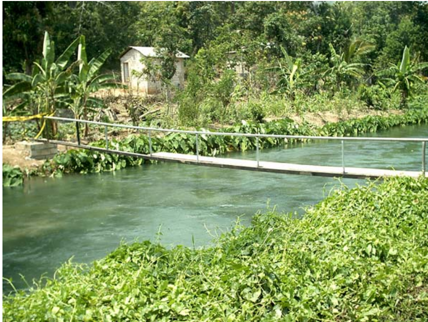
Fig. 3.1. Footbridge placed across canal to enable flow data collection without interfering with flow
