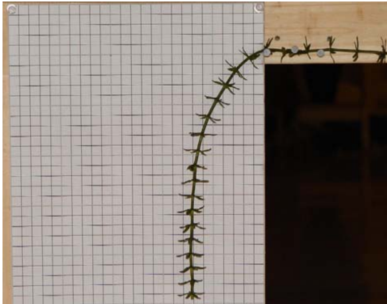
Fig. 5.23b. Bending of same hydrilla stem with 2.9 grams removed from end. (stem and leaves removed)
