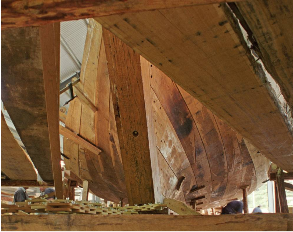
Fig. II.15 The use of temporary cleats on the exterior of the ship's hull to keep the planking in place during the reconstruction of VOC ship Duifje . Photograph: Patrick Baker, Western Australian Museum.
