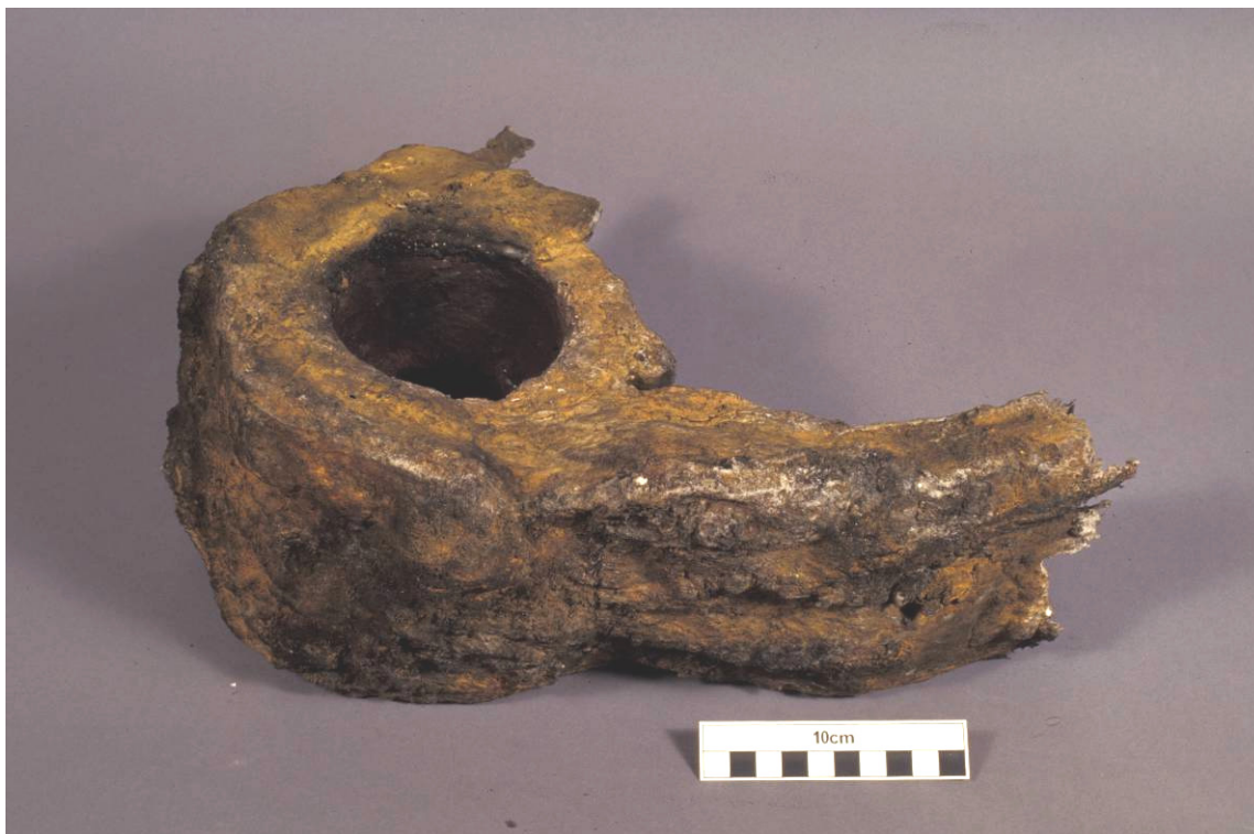
Fig. IV.66 Casting of lower preserved gudgeon from iron concretion, Batavia shipwreck, BAT 80395 R. Photograph: Jon Carpenter, Western Australian Museum.
