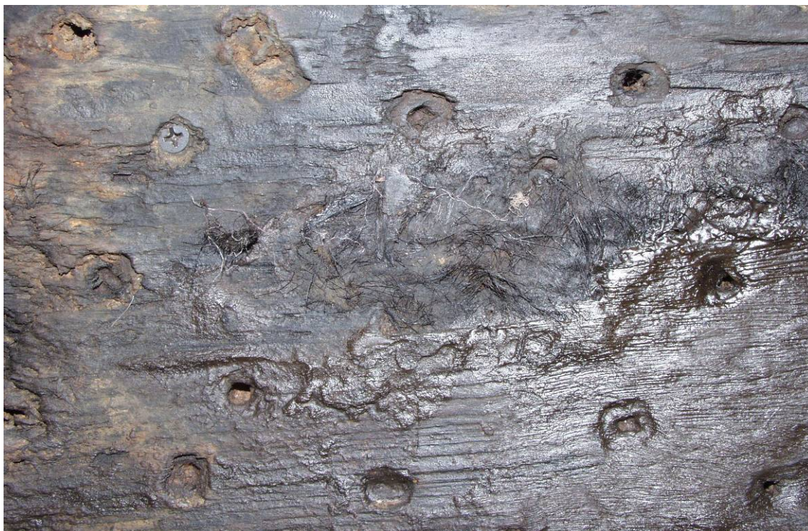
Fig. IV.45 Nail holes with nail head impressions and some goat hair on exterior surface of pine sheathing, Batavia shipwreck, BAT 6241. Photograph: Wendy van Duivenvoorde.
