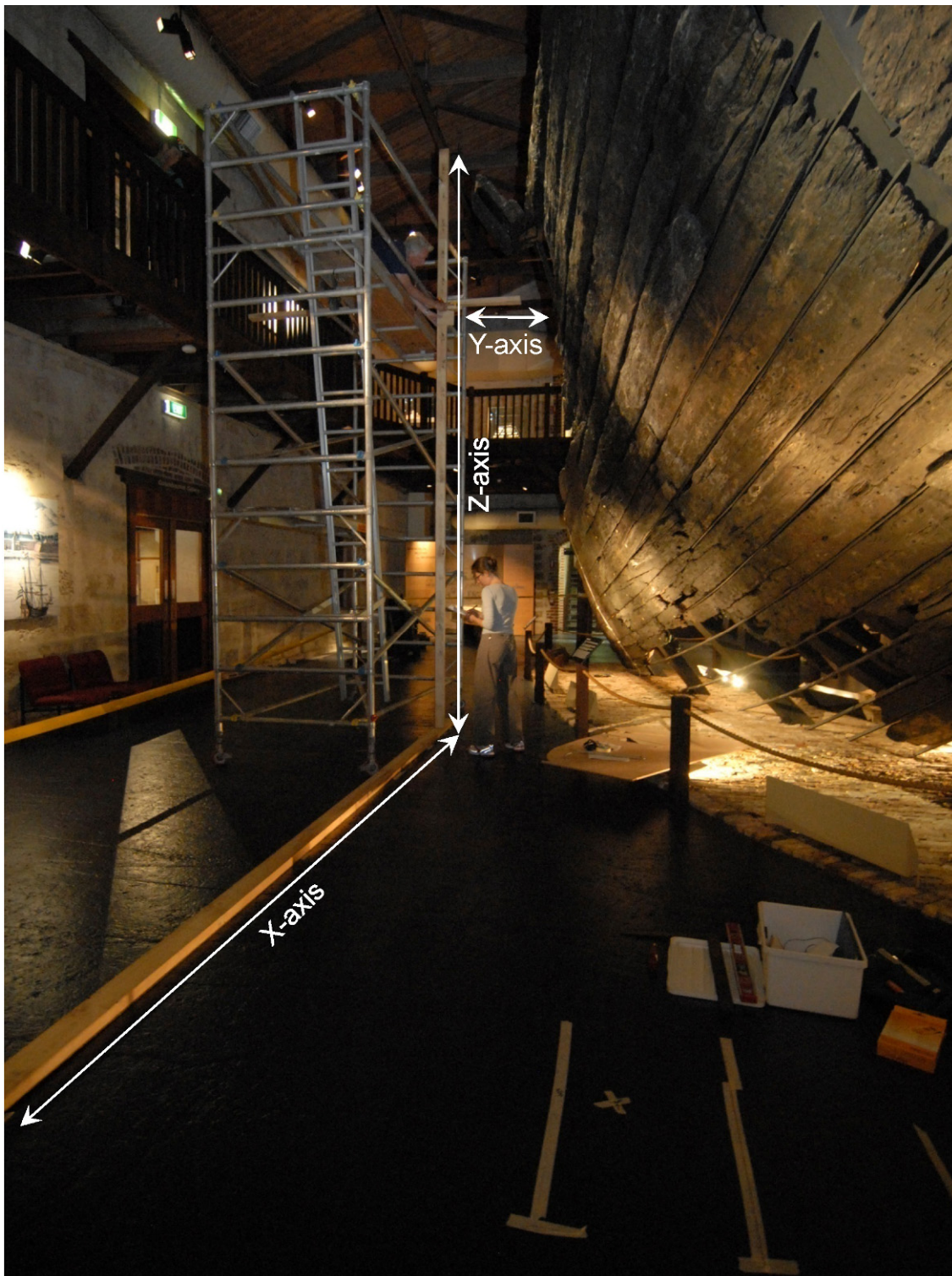
Fig. III.32 Measuring set-up for taking curvatures off Batavia 's hull, showing leveled x-axis and z-axis beams for taking station lines, Shipwreck Galleries of the Western Australian Museum, Fremantle. Photograph: Patrick Baker, Western Australian Museum.
