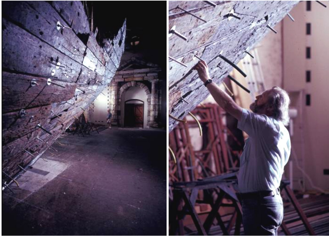
Fig. III.29 Galvanized 16 3 / 4 mm rods were used as screws to hold the planks and frames together, Shipwreck Galleries of the Western Australian Museum, Fremantle. Photograph: Patrick Baker, Western Australian Museum (BT-T-0414, BT-T-0431).
