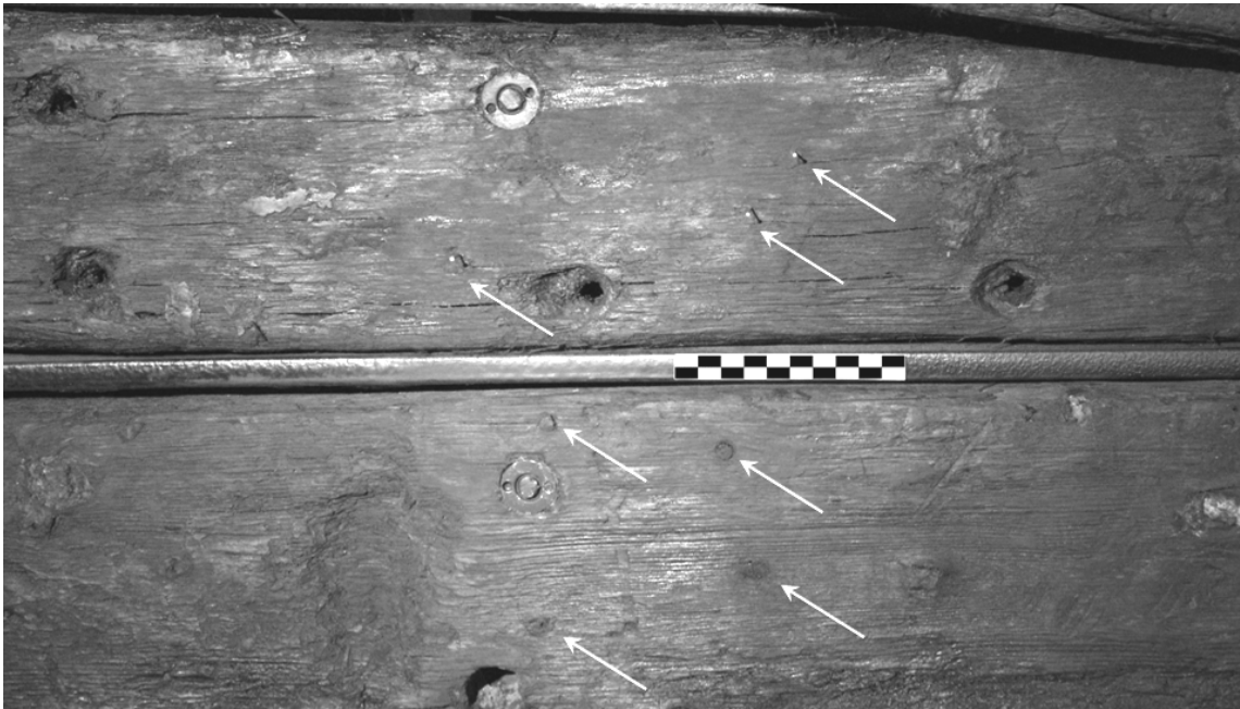
Fig. IV.26 Spijkerpennen or nail plugs on the exterior surface of inner layer of hull planking directly forward of transom, Batavia shipwreck, BAT 6367, Strake 3, and BAT 6390, Strake 4. Photograph: Wendy van Duivenvoorde.
