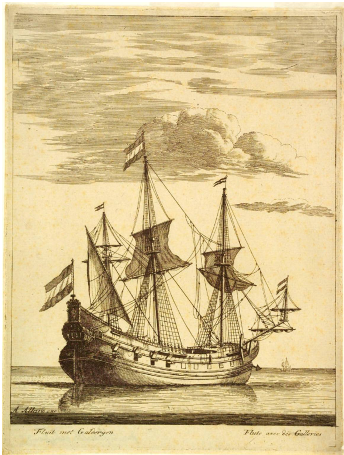
Fig. II.2 Flute ship with narrow upper deck and three wales below the helmsport. Engraving: Abraham Allard, 1650, National Maritime Museum Amsterdam. (A.0149-562).
