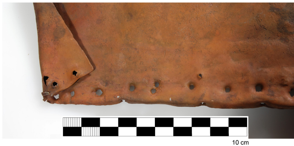
Fig. V.49 Detail showing sheathing nail holes along edge of exterior of outer layer of copper sheet, Vergulde Draak ship's sternpost, GT 3169 A. Photograph: Patrick Baker, Western Australian Museum.
