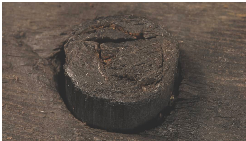
Fig. IV.22 Pegged treenail driven from the inner layer of hull planking, as seen on the exterior surface of the plank, Batavia shipwreck, BAT 6375. Photograph: Patrick Baker, Western Australian Museum.
