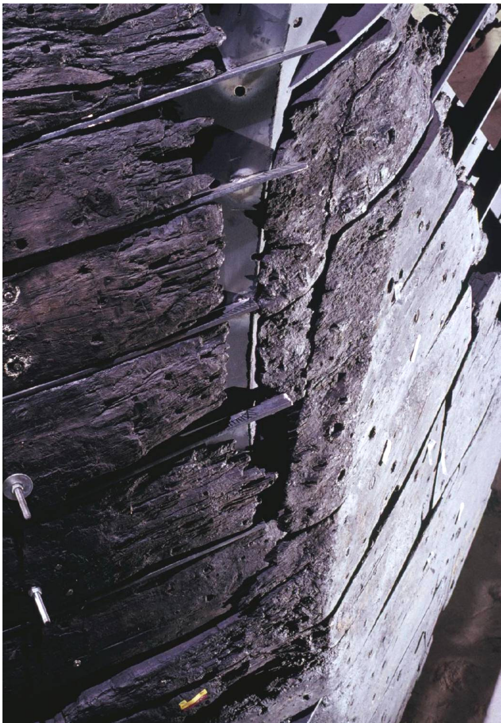
Fig. III.13 Corner of ship's side and transom, showing erosion of the timbers. Photograph: Patrick Baker, Western Australian Museum (BT-T-0455).
