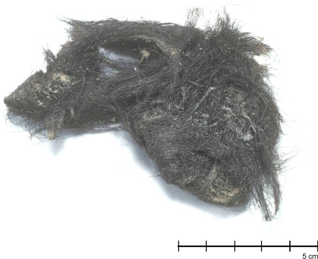
Fig. IV.48 Sample of goat hair from the hair layer between the inner and outer layer of hull planking. Batavia shipwreck, BAT 4123. Photo: Patrick Baker, Western Australian Museum (BT-46-23).
