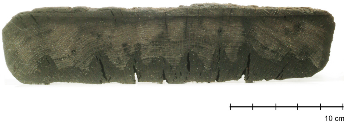
Fig. VII.9 Batavia sample for dendrochronological study, BAT 6180. Cross-section of tangential-sawn oak hull plank. Photograph: Patrick Baker, Western Australian Museum.
