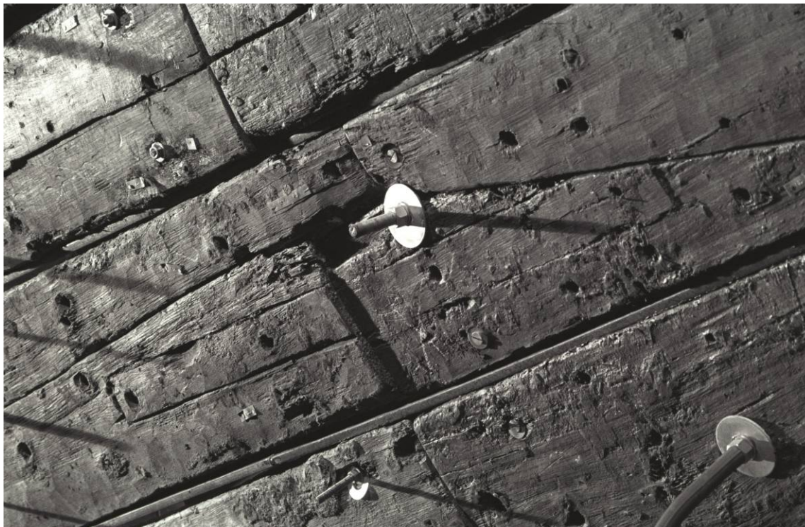
Fig. IV.32 Rectangular graving piece forward of scarf end on exterior of inner layer of hull planking, sawn in two sections during excavation, Batavia shipwreck, BAT 6206 and BAT 6074, Strake 11. Photograph: Patrick Baker, Western Australian Museum (MA4068–10).
