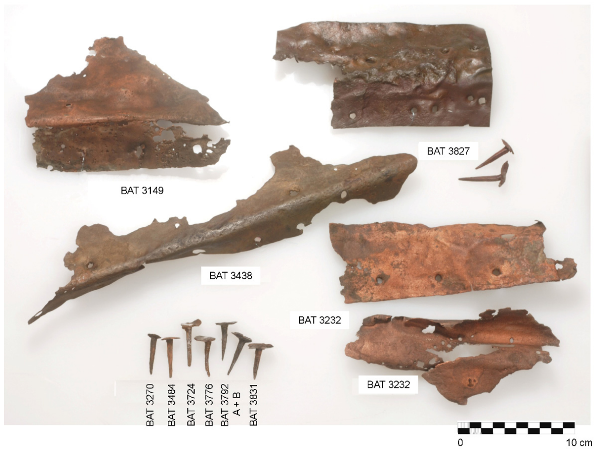
Fig. IV.69 Fragments of copper sheathing and tacks from sternpost, Batavia shipwreck. Photograph: Patrick Baker, Western Australian Museum.
