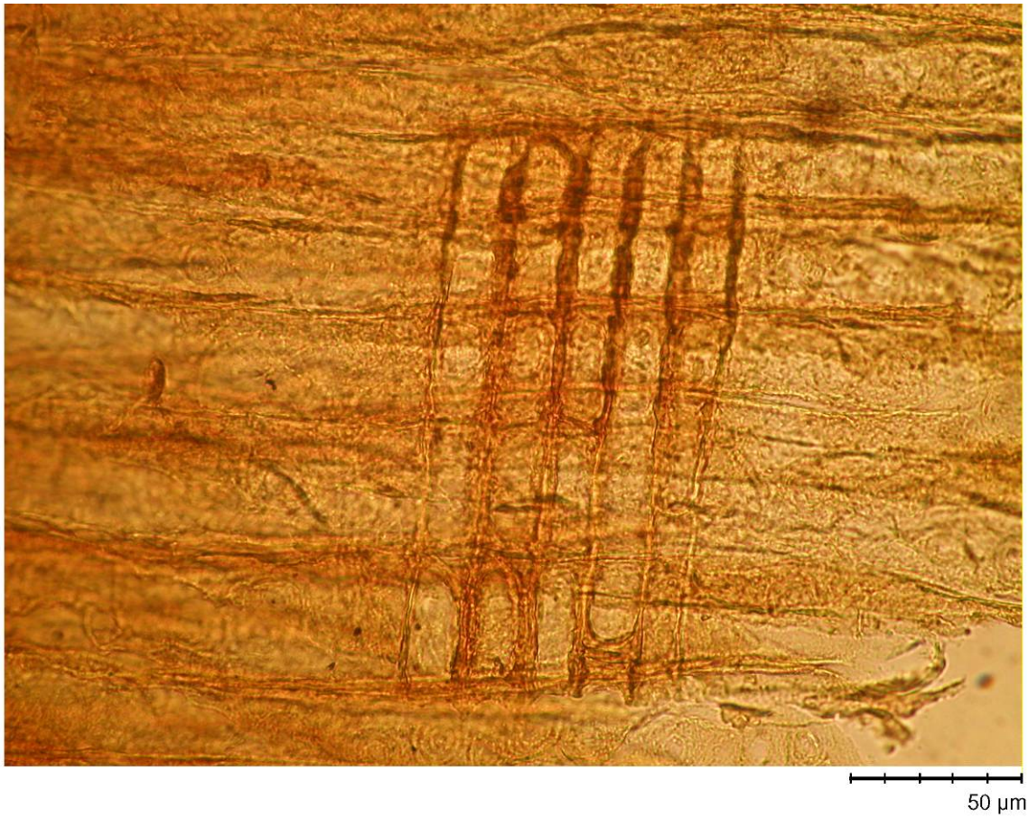
Fig. VII.6 Radial section with parenchyma cells with large open pits, mostly one per cross field. Pinus sp. Batavia shipwreck, BAT 6150. Dissecting microscope, magnification x400. Micrograph: Mark van Waijjen, BIAAX Consult.
