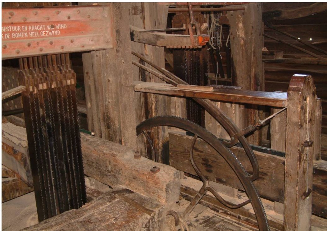
Fig. V.39 Sawing blades of a still operational wind-driven sawing mill (originally built prior to 1683), De Rat , in IJlst, Netherlands. Photograph: Simon Jellema, miller of De Rat .
