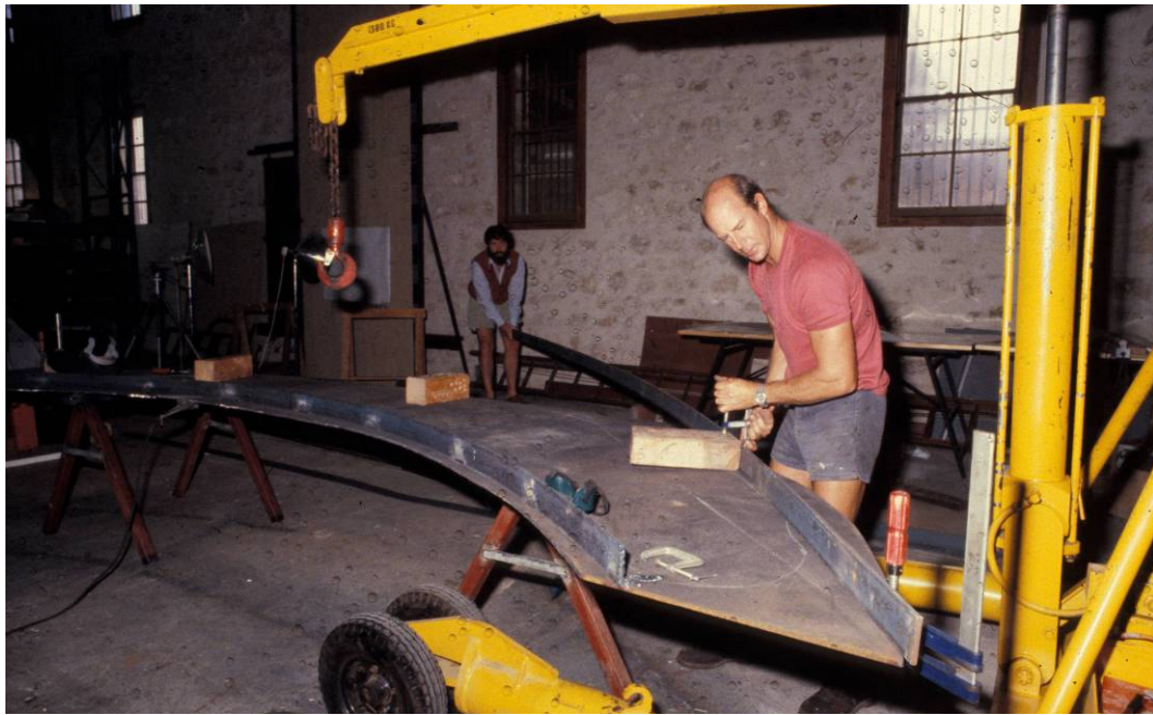
Fig. III.23 Geoff Kimpton (right) and Jeremy Green (left) constructing the steel backing plate for Batavia 's fashion piece. Photograph: Brian Richards, Western Australian Museum (BT-T-0100).
