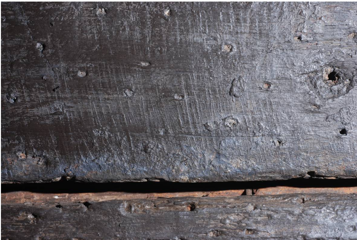
Fig. IV.88 Outer hull planking with saw marks of framed pit saw, Batavia shipwreck, BAT 6078 (top), Strake 13. Photograph: Patrick Baker, Western Australian Museum.
