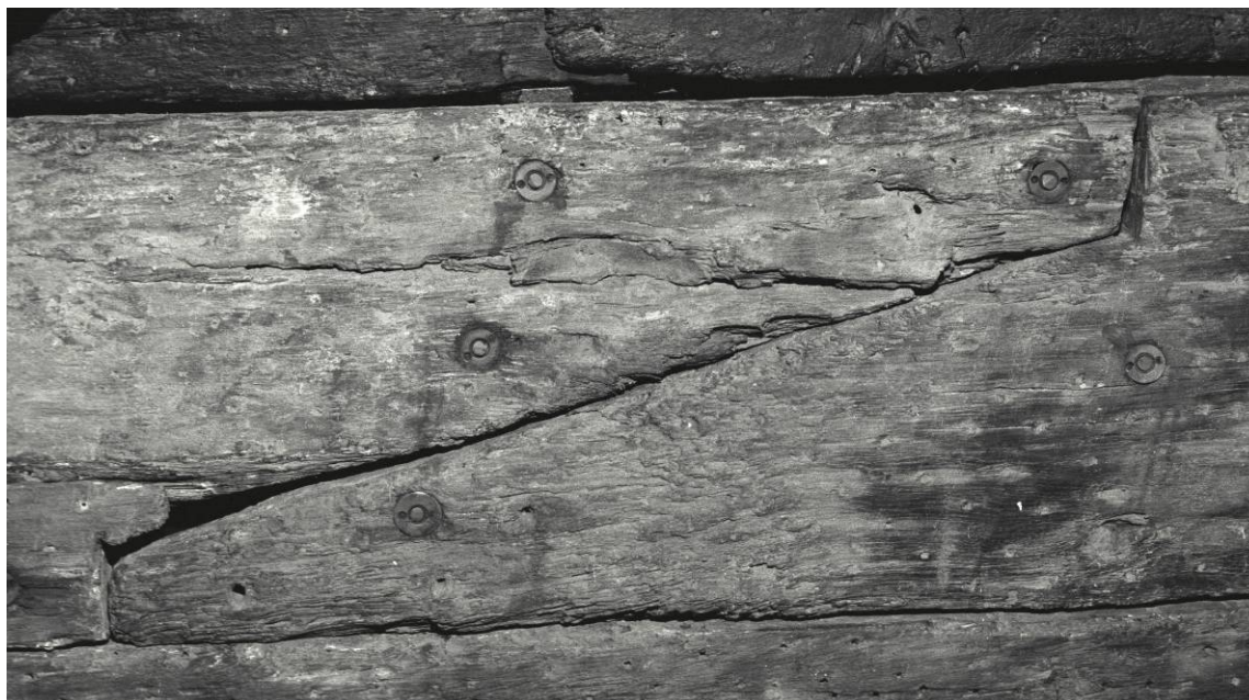
Fig. IV.18 Flat scarf in planking strake 12, exterior of outer layer of hull planking, Batavia shipwreck, BAT 6014 and BAT 6106. Photograph: Patrick Baker, Western Australian Museum (MA4864-34).
