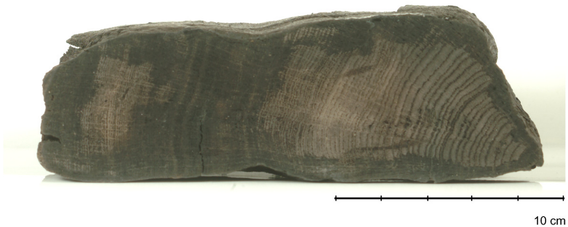
Fig. VII.11 Batavia sample for dendrochronological study, BAT 6375. Cross-section of tangential-sawn oak hull plank over tree's center. Photograph: Patrick Baker, Western Australian Museum.
