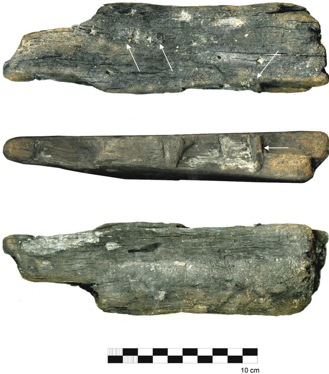
Fig. V.33 Fragment of hull planking of VOC ship Vergulde Draak , GT 6142 P, location of nail plugs indicated by arrows. Photograph: Wendy van Duivenvoorde.
