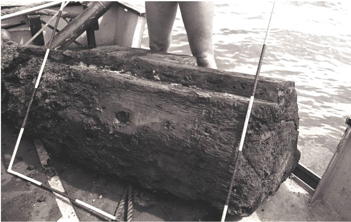
Fig. IV.77 Chamfered after surface of wing transom with rabbet to receive transom planking (timber is lying upside down), Batavia shipwreck, BAT 6369. Photograph: Patrick Baker, Western Australian Museum (MA0414–15).
