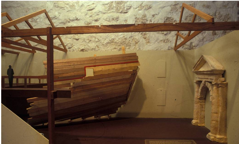
Fig. III.21 1:10 scale model of the initial design for the reassembly of the Batavia hull. Photograph: Patrick Baker, Western Australian Museum (BT-T-0164).
