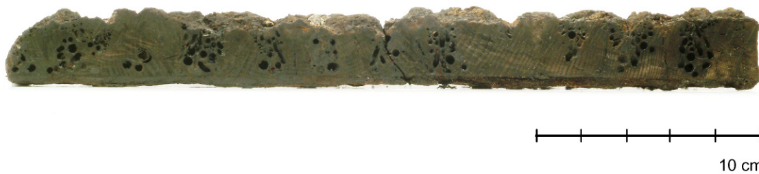
Fig. VII.12 Batavia sample for dendrochronological study, BAT 6441. Cross-section of tangential-sawn pine sheathing with wormholes. Photograph: Patrick Baker, Western Australian Museum.
