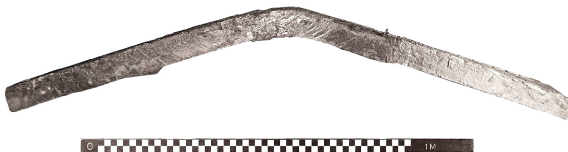
Fig. IV.40 Saw marks on edge of transom plank, Batavia shipwreck, BAT 6417. Photograph: Patrick Baker, Western Australian Museum (MA0422–32).
