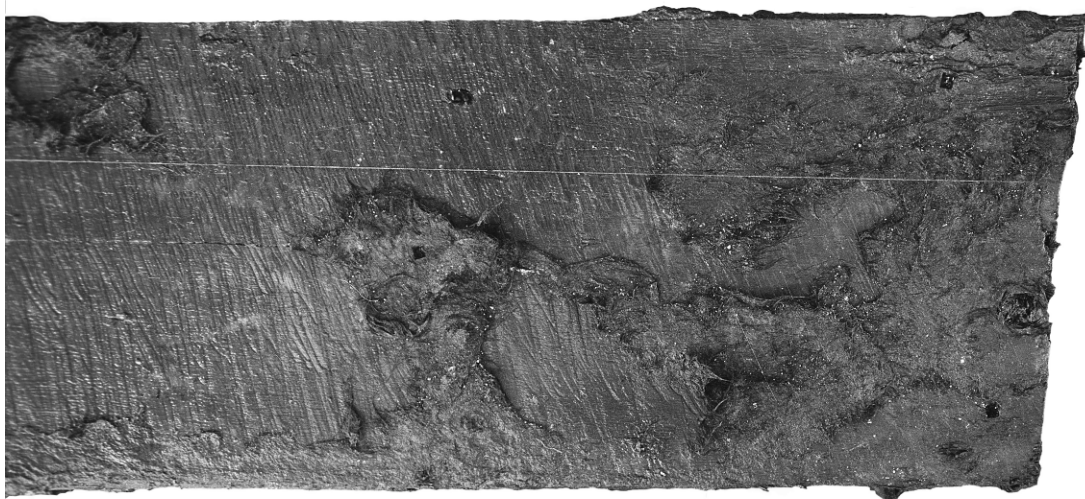
Fig. IV.87 Saw marks of framed pit saw on interior surface of outer hull planking, Batavia shipwreck, BAT 6106, Strake 12. Photograph: Patrick Baker, Western Australian Museum (MA0188-26).
