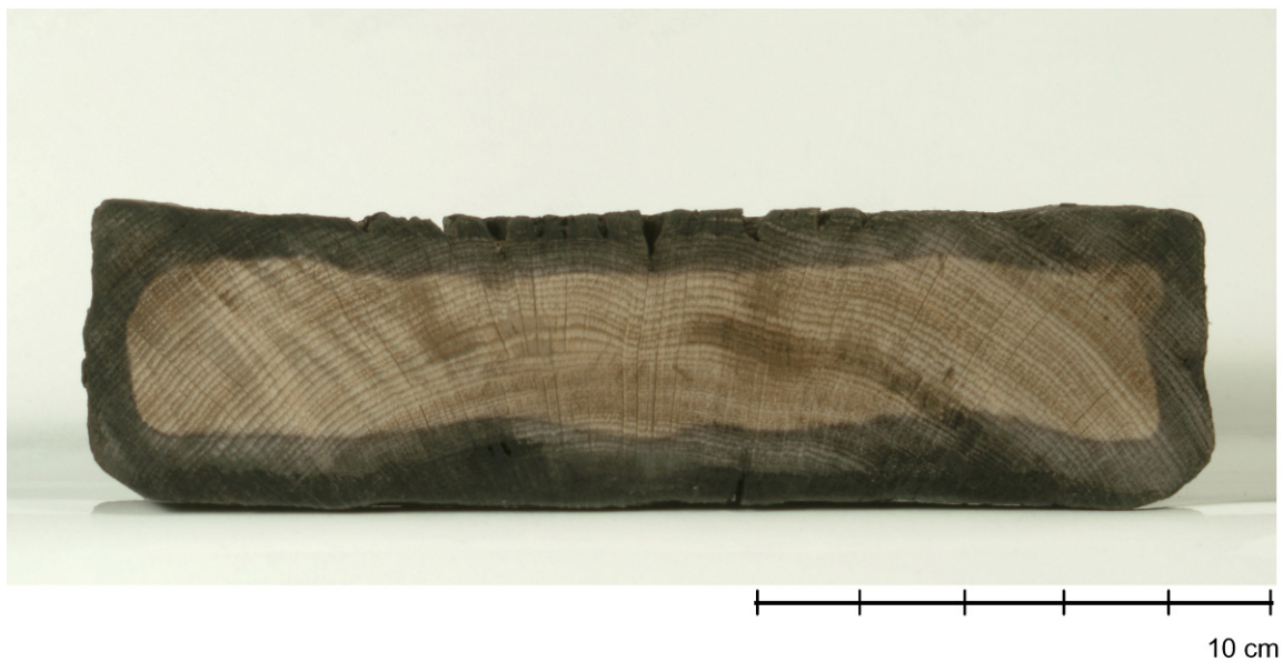
Fig. VII.10 Batavia sample for dendrochronological study, BAT 6226. Cross-section of tangential-sawn oak hull plank. Photograph: Patrick Baker, Western Australian Museum.
