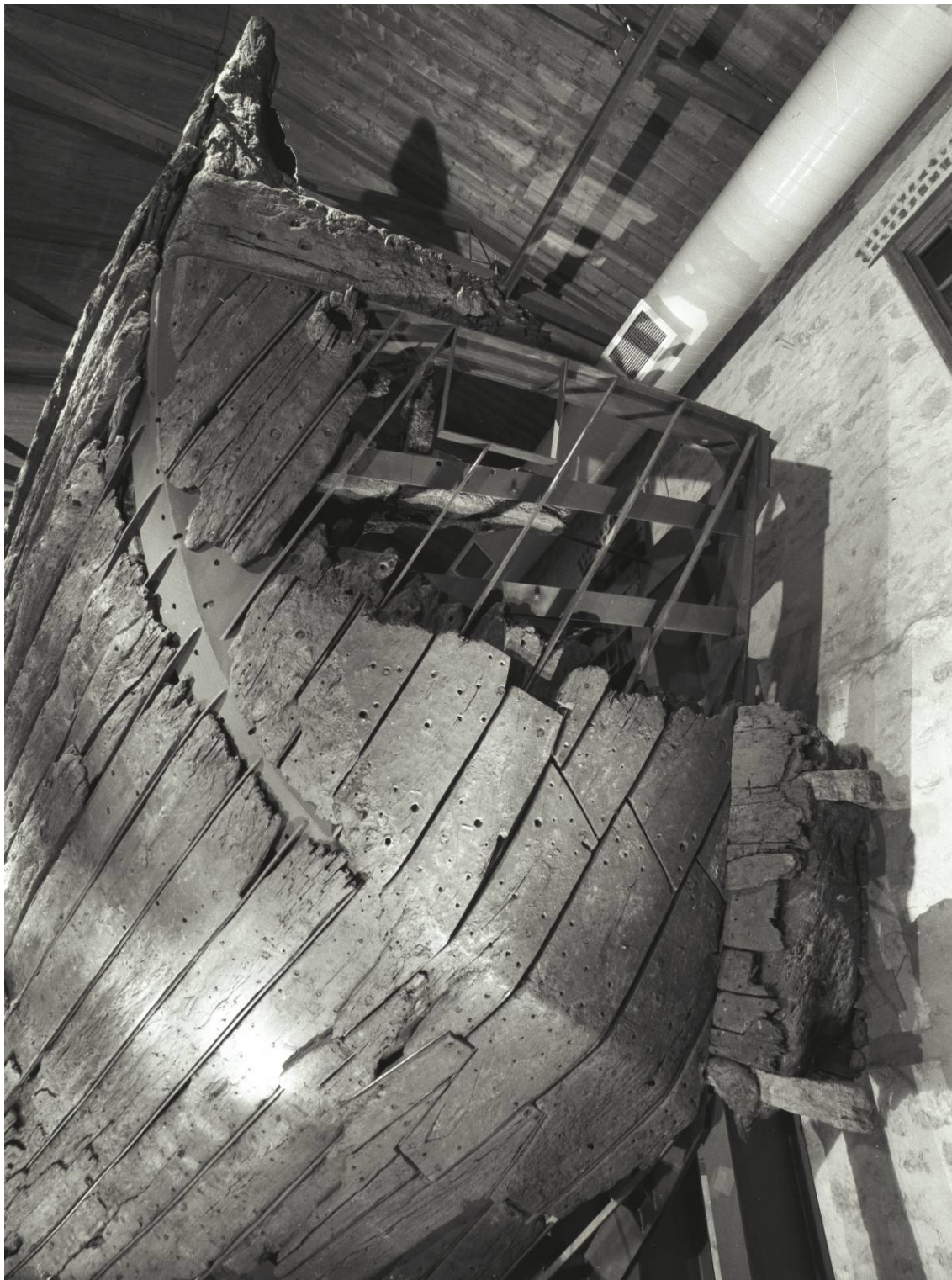
Fig. IV.34 Batavia's port side transom planking and sternpost. Photograph: Patrick Baker, Western Australia Museum (MA5048–30).
