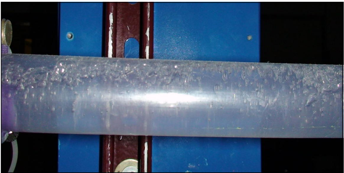
Fig. 3.5 – Aerated liquid flow without flow conditioners.
