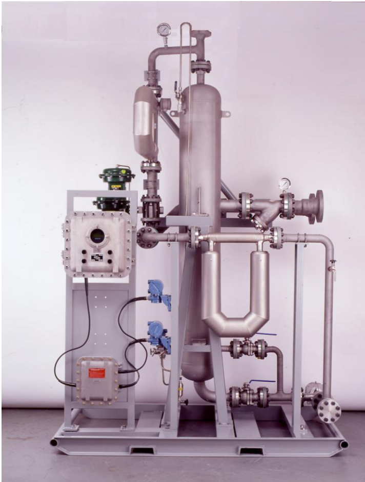
Fig. 1.4 – Multiphase metering system using compact separation and Coriolis meters (from Phase Dynamics).
