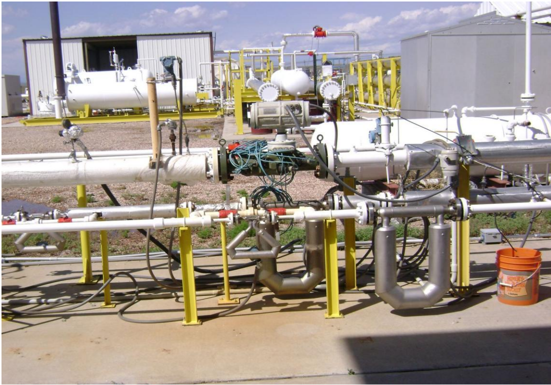
Fig. 2.3 – U-tube Coriolis meter in use for calibration of other meters at CEESI, Colorado.
