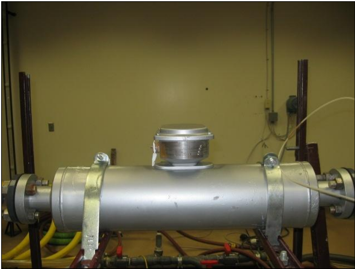
Fig. 3.2 – Single straight tube Coriolis meter used in experiments.
