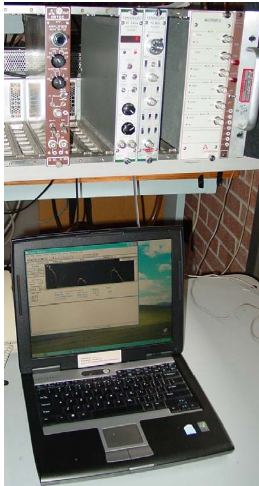
Figure 2.18. Acquisition system. Top: multichannel analyzer, Multiport II. Bottom: portable computer with Genie 2000® software.
