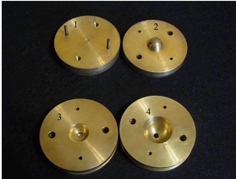
Figure 2.8. Mold parts. Top: disk with two stainless steel rods and solid brass disk with a central protuberance. Bottom: two cylindrical sets of brass disks.
