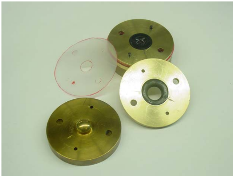
Figure 2.9. Preassembled hemisphere. The whole set of plastic/brass disks corresponding to a hemisphere will be stacked, lying polyethylene layers between them to provide electrical isolation.
