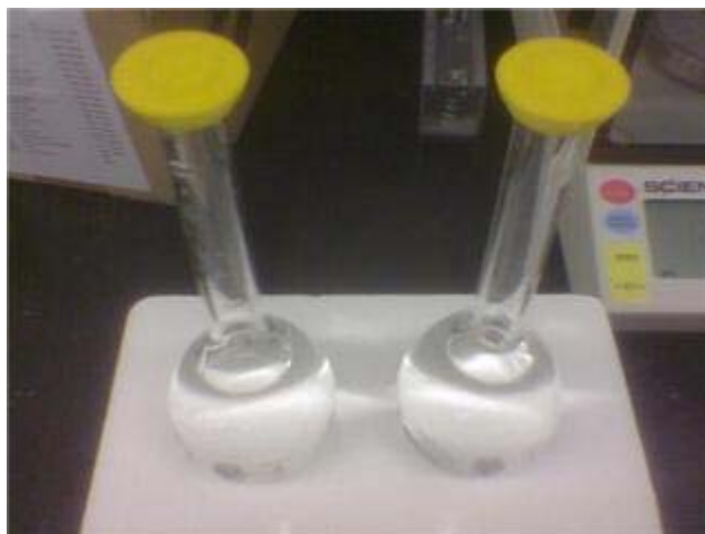
Figure 16. Initial phenanthroline mixing errors led to no color development within solutions.
