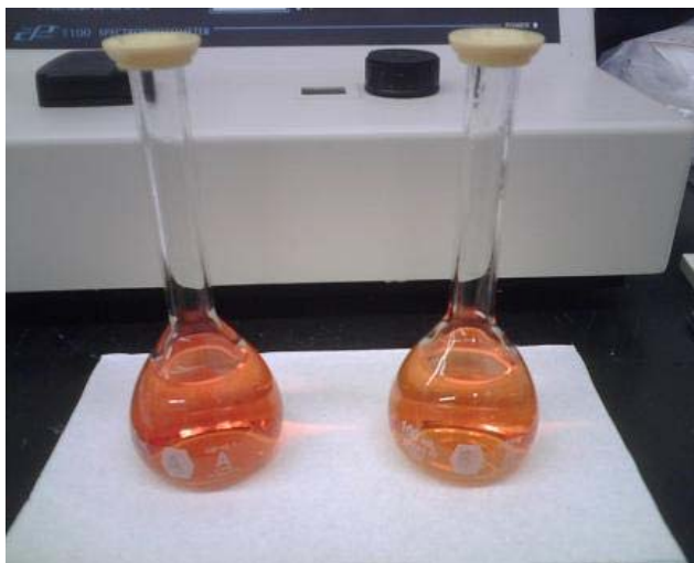
Figure 17. Proper color development following corrections to initial phenanthroline procedure.
