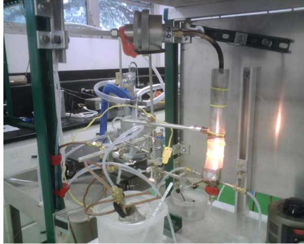
Figure 6. New soot collection system.
