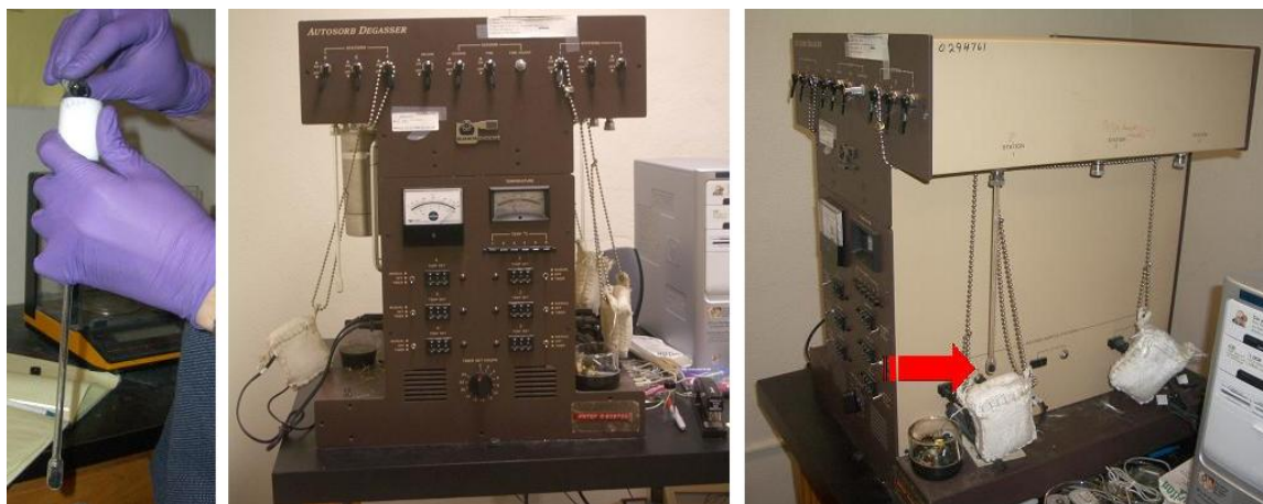
Figure 8. Soot sample preparation (left); front of degasser (middle); cell inserted with heated bag below (right).
