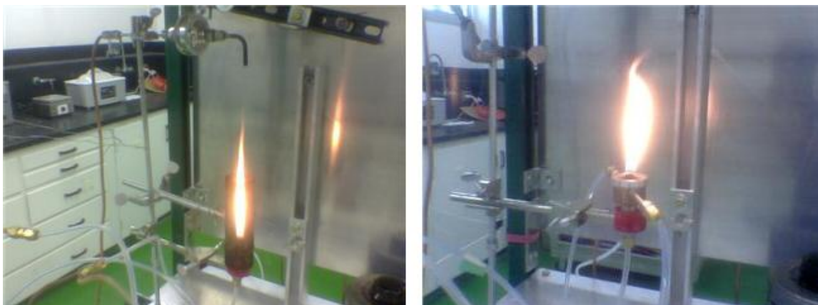
Figure 4. Initial soot generation setup with co-flow head (left); flame without co-flow head.
