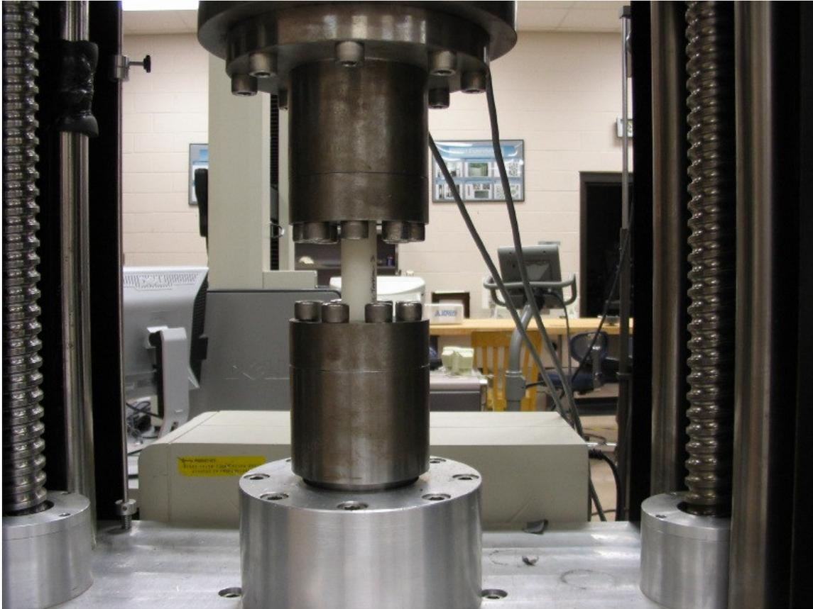
Fig. 7. Close up of the torsion test
