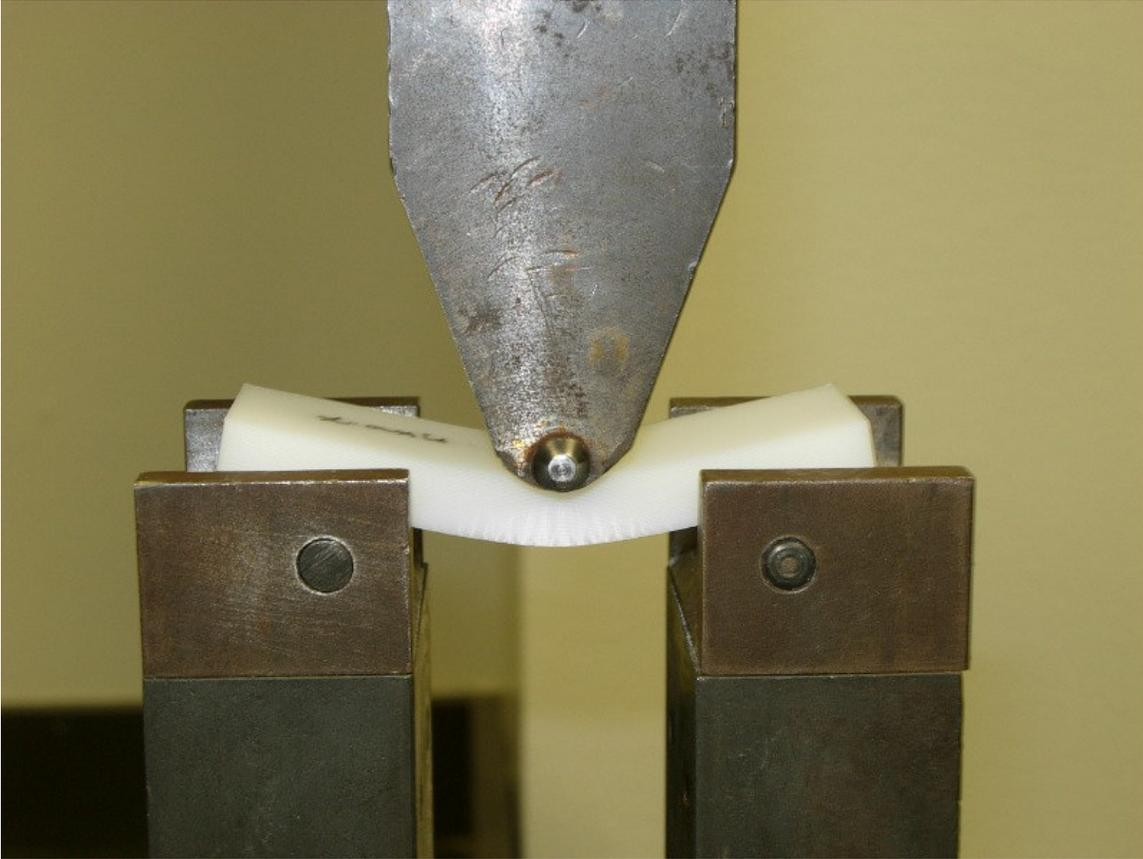
Fig. 33. Close up of a specimen undergoing three-point bending
