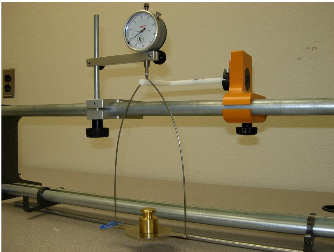
Fig. 48. Close up of the dial gauge, specimen and the weight pan
