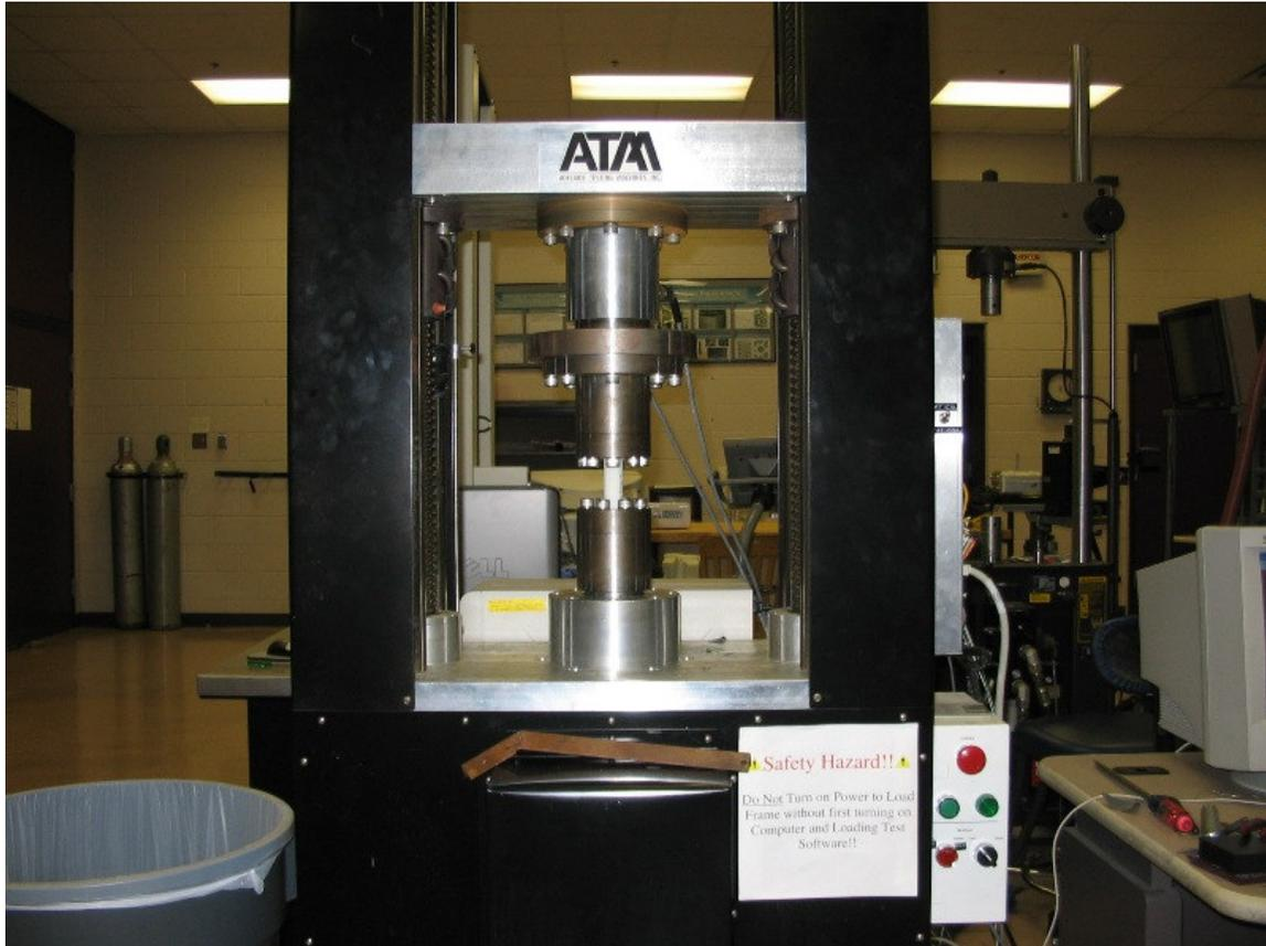
Fig. 5. The Adelaide load frame on which torsion tests were conducted
