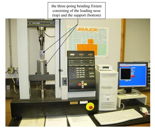
Fig. 32. The Instron 4411 load frame on which the three-point bending tests were conducted
