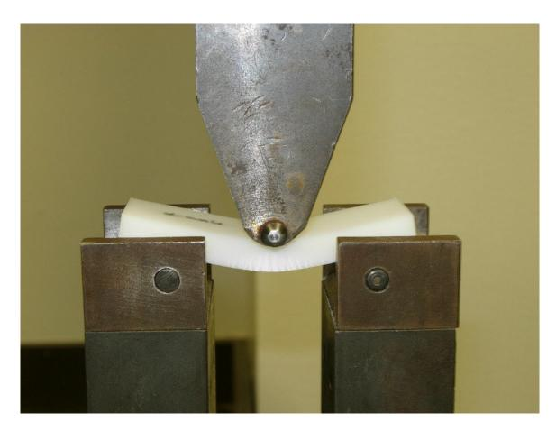
Fig. 33. Close up of a specimen undergoing three-point bending
