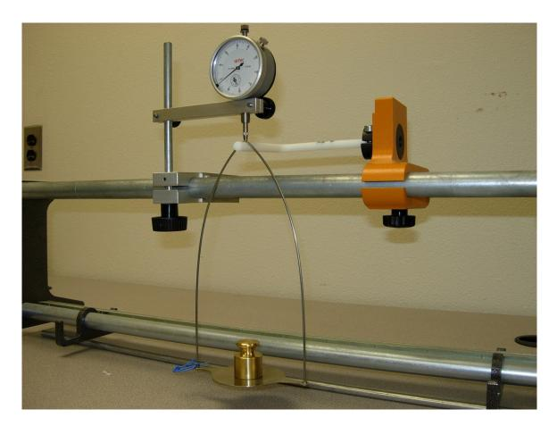
Fig. 48. Close up of the dial gauge, specimen and the weight pan
