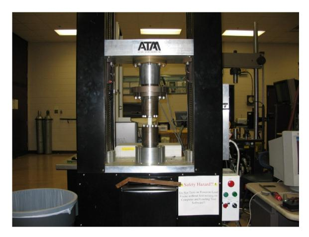
Fig. 5. The Adelaide load frame on which torsion tests were conducted
