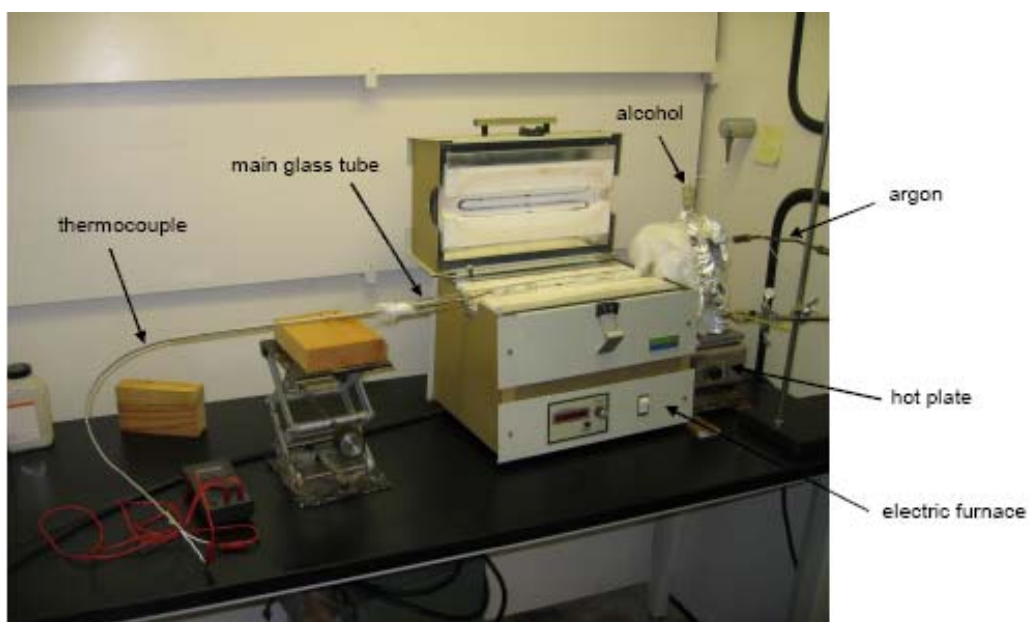
Figure 9. CVD System (Courtesy of S.K. Sinha, UNH)
