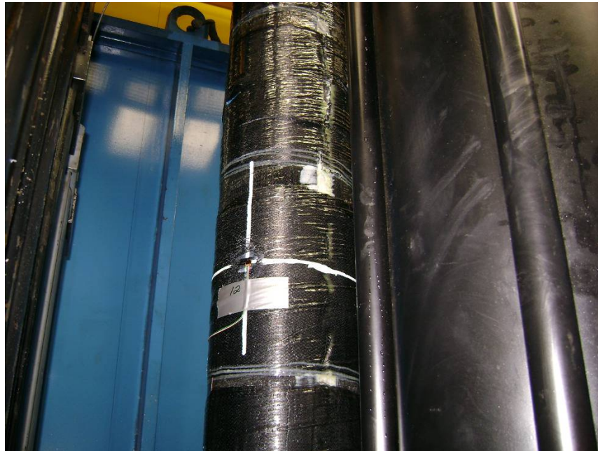
Figure 70 – Photo of tension test showing fracture
