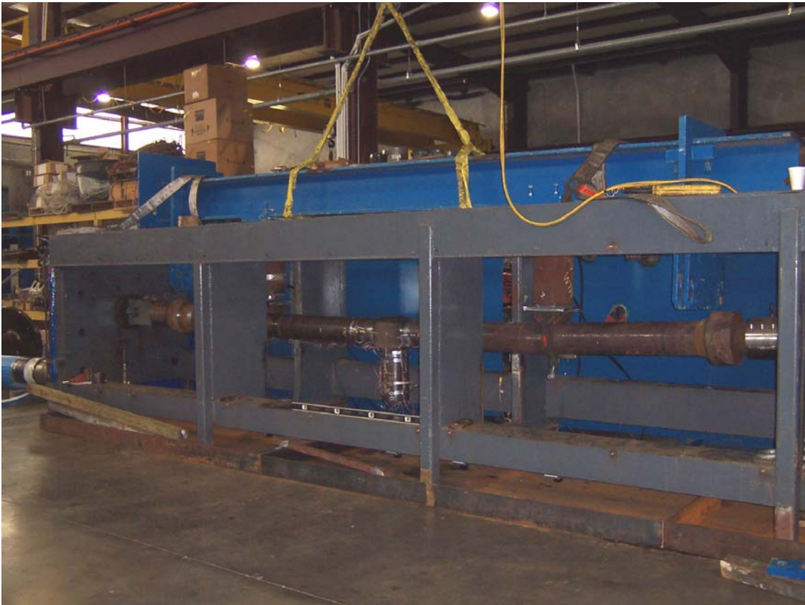
Figure 9 – Load frame used for pressure-tension-bend testing
