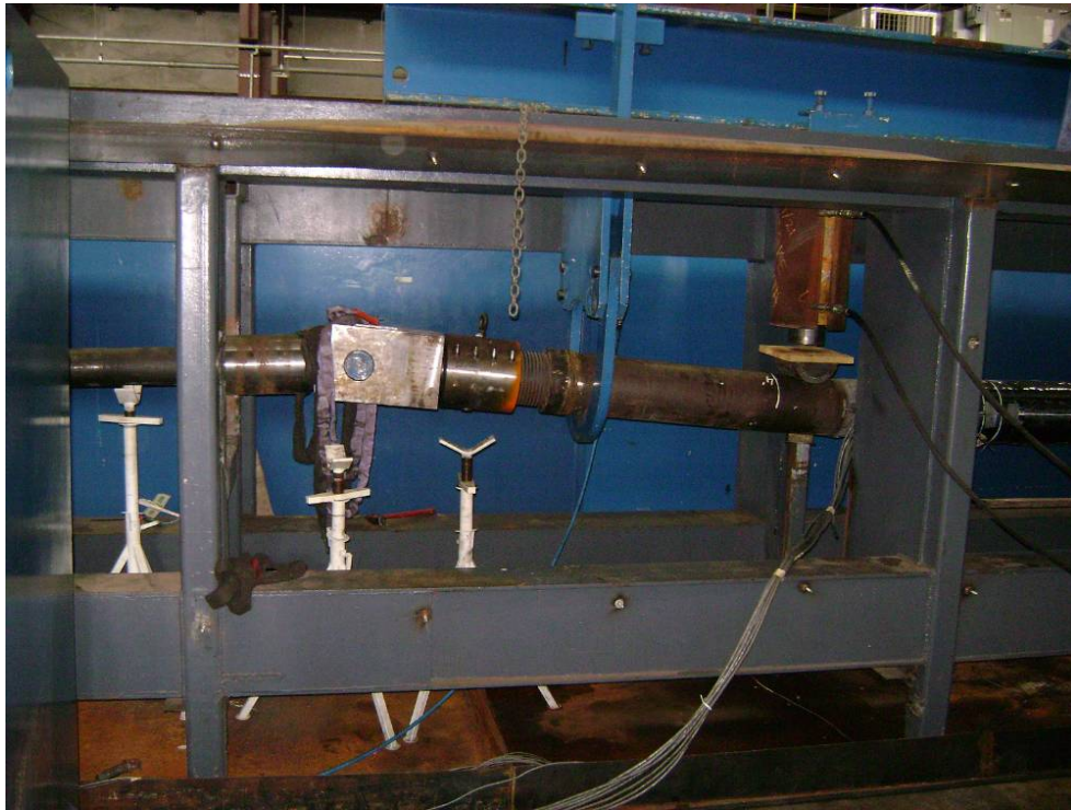
Figure 72 – Photograph showing displaced configuration of bending sample
