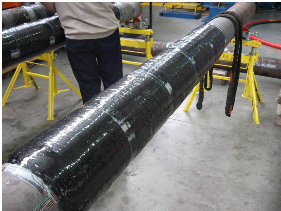
Figure 55 – Final view of cured repair prior to testing
