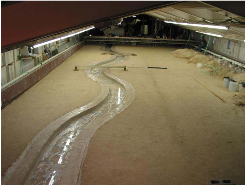
Figure B.4 Initial Condition of Clay Test Case 03 ( R/W = 6 , \phi = 65^\circ , Fr = 0.50 )
