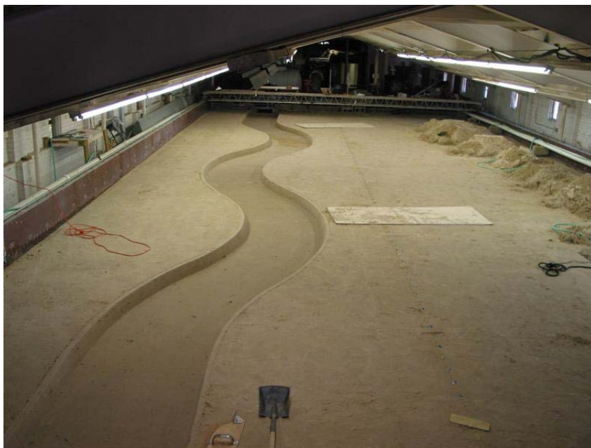
Figure A.6 Digging the Sand Channel
