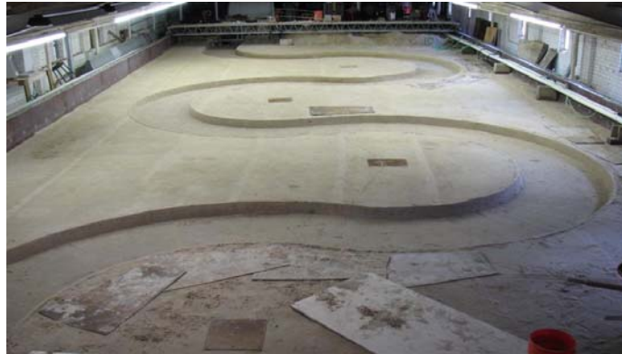
Figure 4.18 Carved Guide Channel in the Sand Bed
