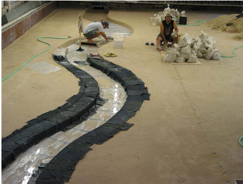
Figure A.7 Placing the Clay Banks and Covering with Wet Cloth
