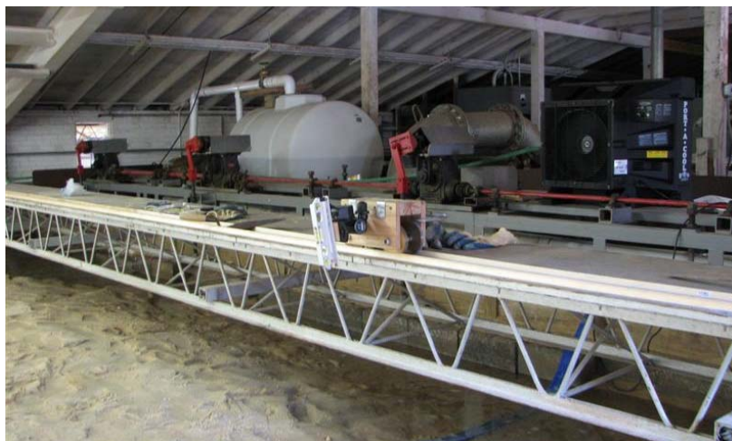
Figure 4.11 Carrier with Laser Sliding on the Bridge for Transverse Coordinate (y-direction) Measurement
