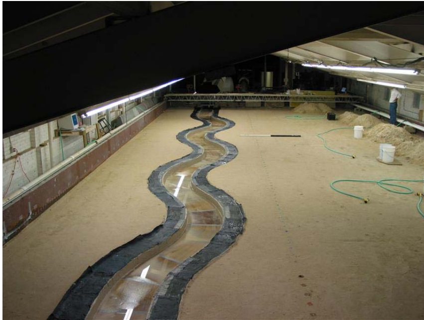
Figure B.6 Initial Condition of Clay Test Case 04 ( R/W = 4 , \phi = 65^\circ , Fr = 0.50 )
