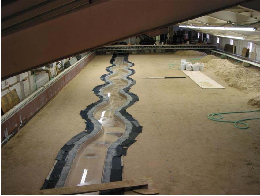
Figure B.10 Initial Condition of Clay Test Case 06 ( R/W = 2 , \phi = 65^\circ , Fr = 0.50 )
