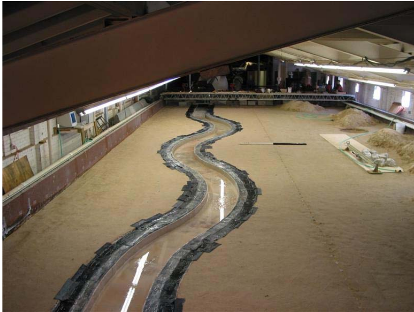
Figure B.8 Initial Condition of Clay Test Case 05 ( R/W = 6 , \phi = 65^\circ , Fr = 0.50 )
