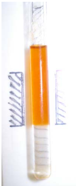
Figure II-2. A suspension of O-am-[A] in CDCl 3 for NMR spectroscopy. It is aligned with a drawing provided by the TAMU NMR facility showing the location of the magnetic field with respect to the sample.
