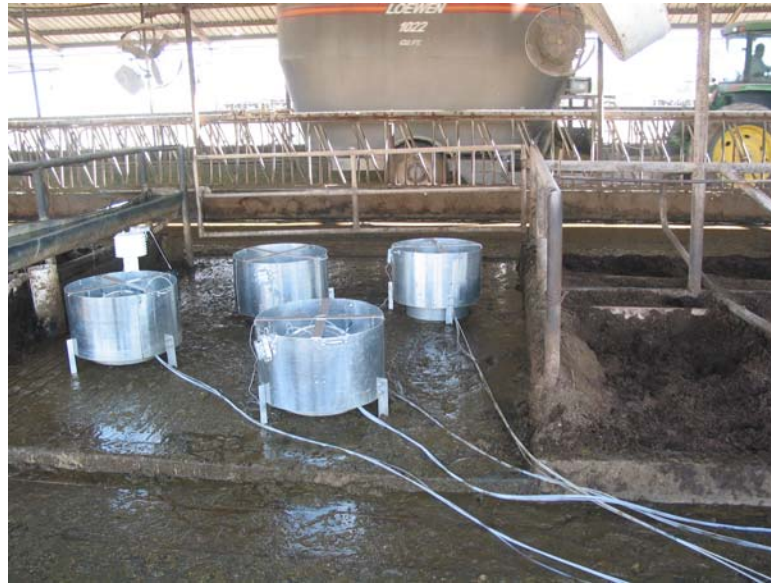
Figure 4.3. Isolation flux chambers in a free-stall barn.
