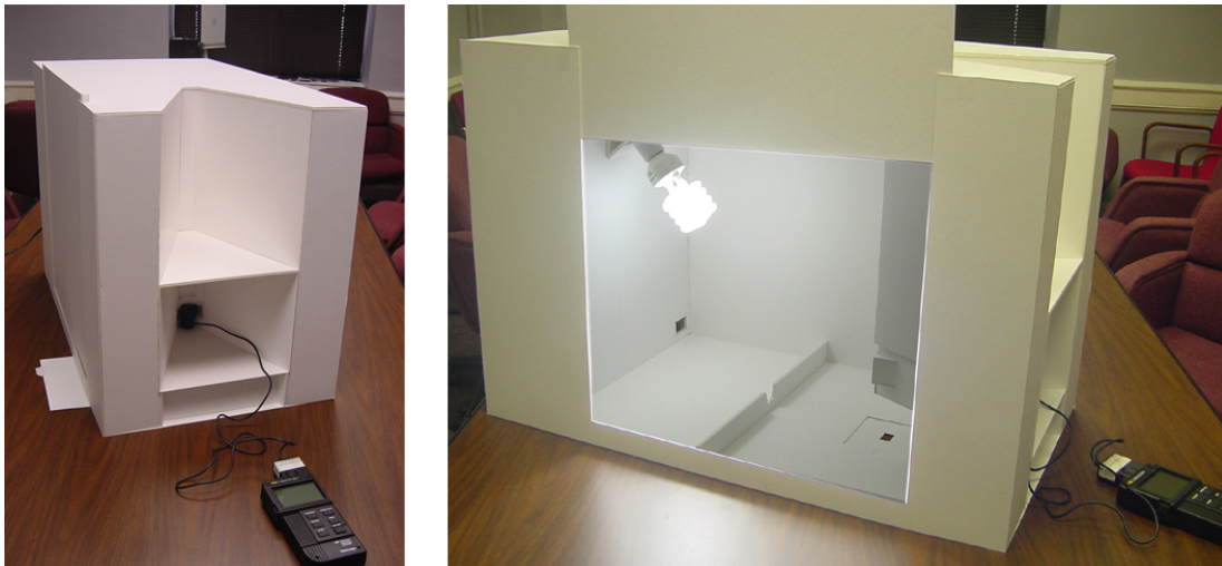
Figure 5.7: Measurement of Color Quality Printed on Matt Paper in Isolation
