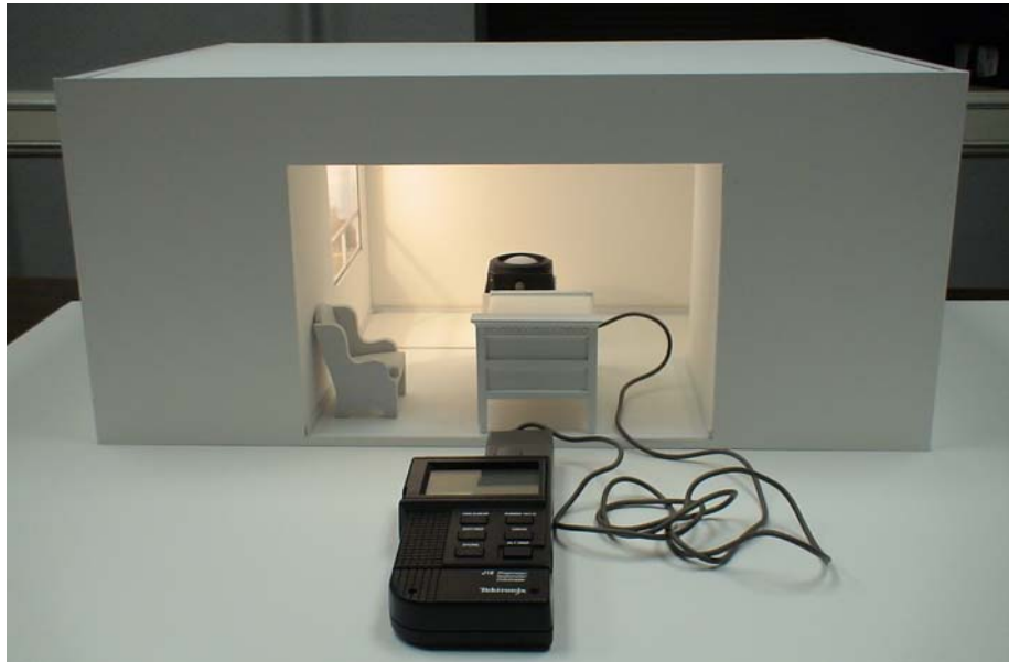
Figure 5.1: Illuminance Measurement Method inside Scale-Models
