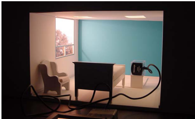
Figure 5.8: Measurement of Visual Quality of Color in Scale-Model
