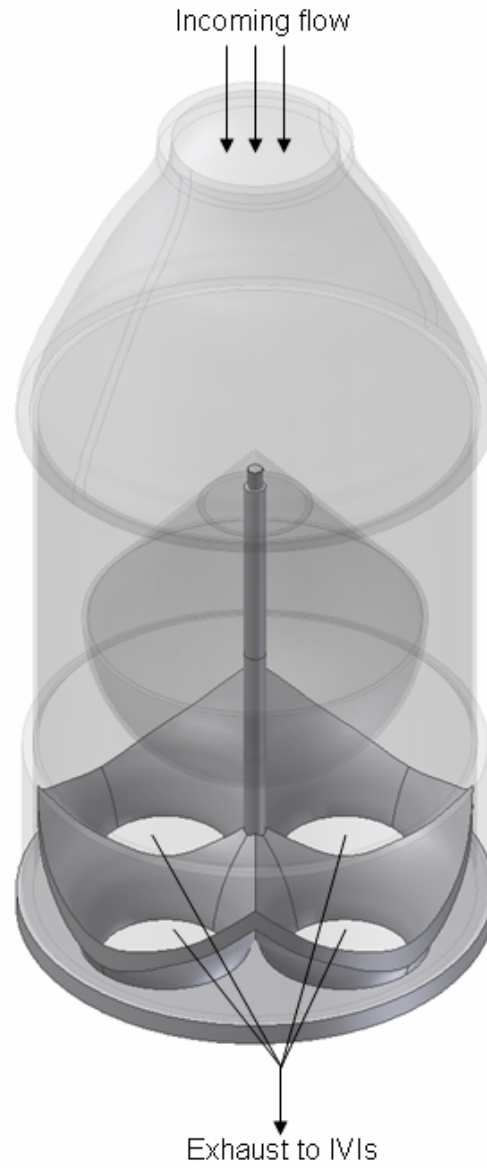
Figure 6.5. Inlet manifold used for distribution of aerosol to four IVI-350 units
