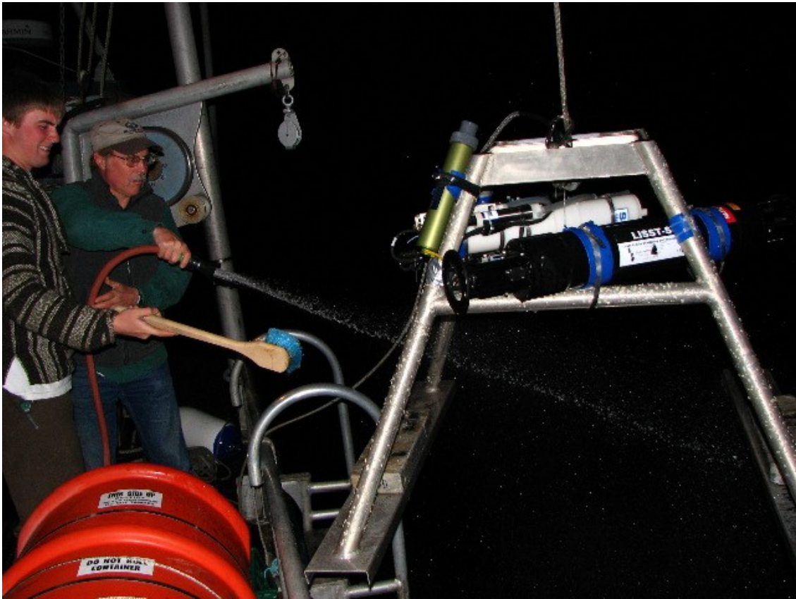
Fig 18 Picture of the instrumented pod. The pod was tethered to a surface line with float for retrieval
