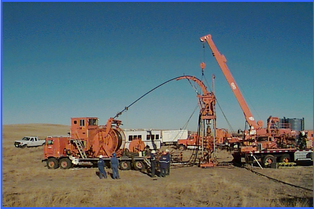
Fig. 2.9a: A coiled tubing truck involved in a fracturing operation ( source: Schlumberger )
