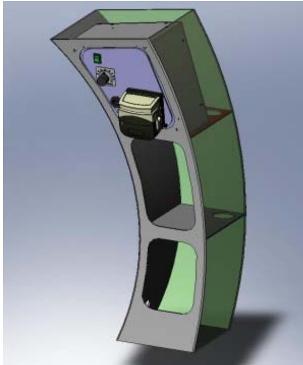
Fig. 8. Estimating fit using three dimensional models of the pump and Bovie Cart.
