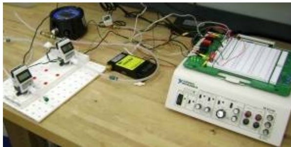
Fig. 10. Pressure and flow instruments connected to the data acquisition system.
