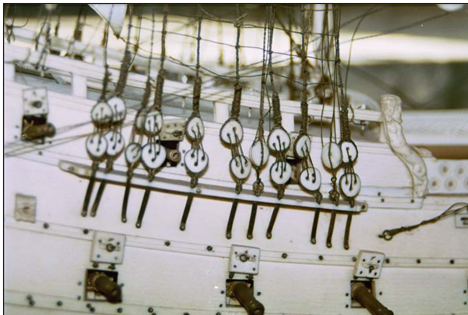
Fig. 62. Norske Løve (1654), deadeye straps in the mizzen channel. (C. Corder)
