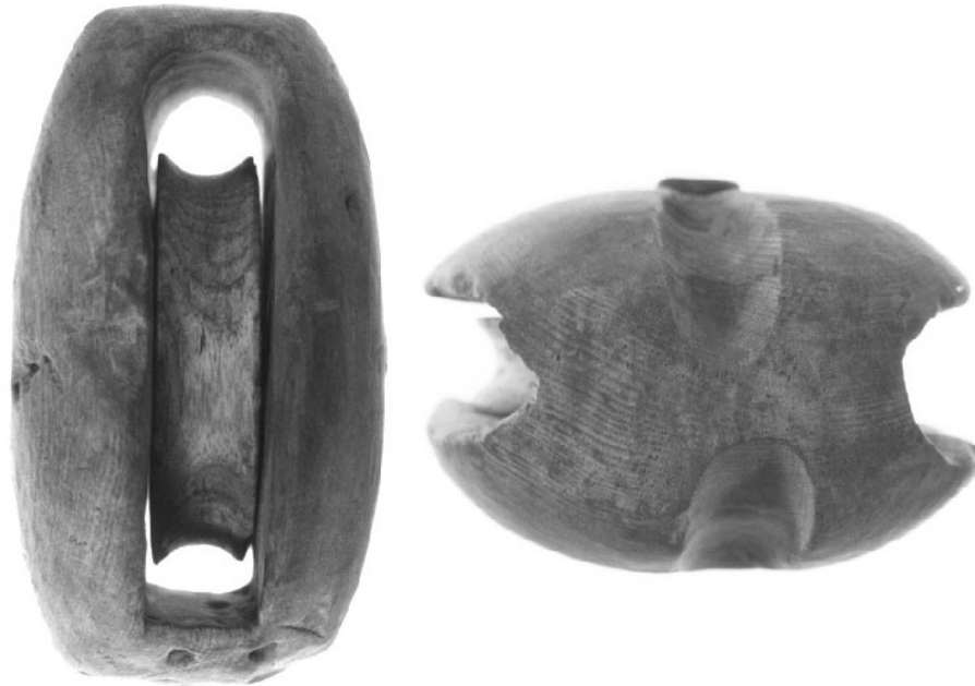
Fig. 4. Block 3326 from La Belle : channel and feed (left); exterior of shell with incomplete scoring (right). (C. Corder)
