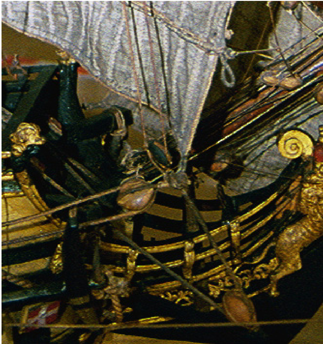
Fig. 37. Sheet, clew garnet, and tack on the forecourse bonnet of the Danish Church Model (ca. 1680) in Orlogsmuseet. (C. Corder)
