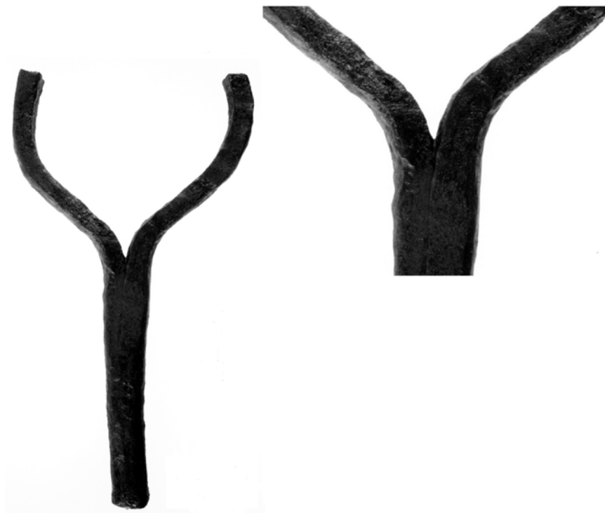
Fig. 29. A topmast deadeye strap and partial futtock plate, artifact 12576 from La Belle , demonstrating the visible seam at the deadeye strap's neck as it transitions from square to round in cross-section. (C. Corder)
