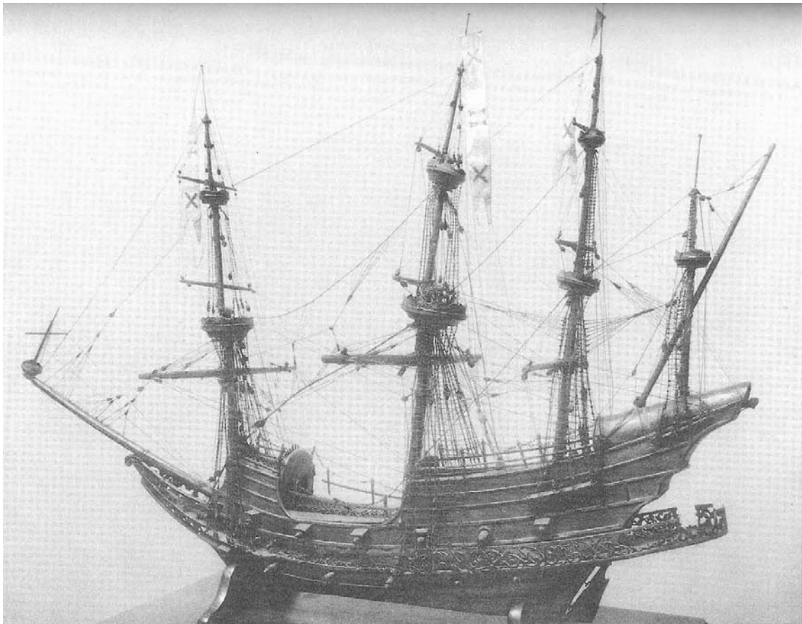
Fig. 47. These church models exaggerate the forward-raking foremast and aft-raking mizzen mast common to the 16th and early 17th centuries. (Nance 2000, pls. 9, 10)
