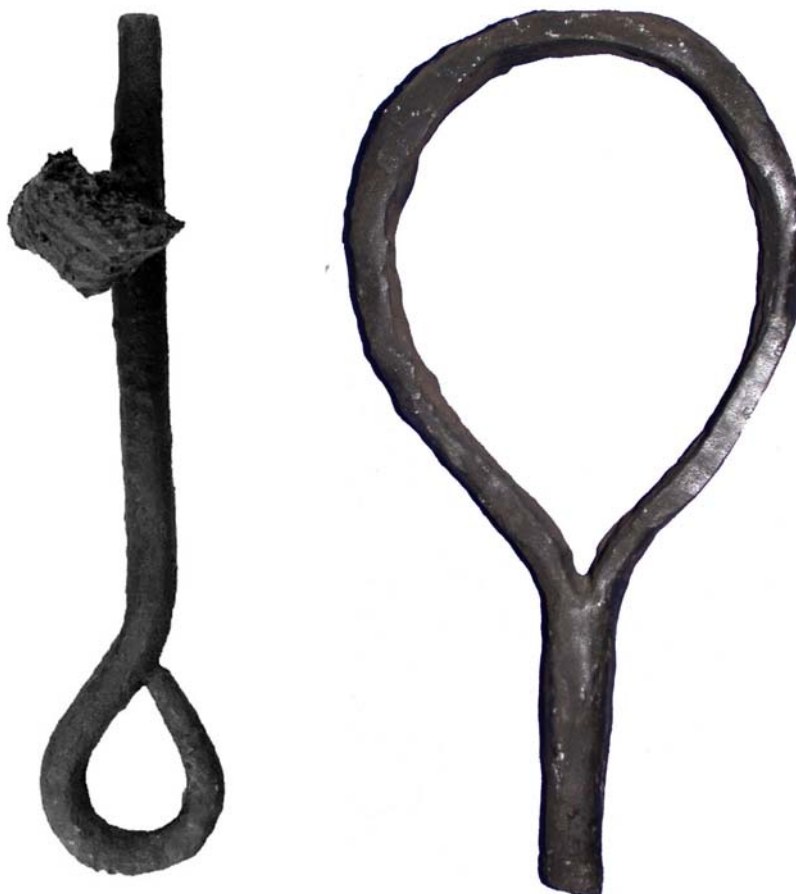
Fig. 30. A futtock plate (left, 2004), and topmast deadeye strap (right, 6013) from La Belle . Futtock plate 2004 demonstrates the type that was once attached to the deadeye strap at right. (C. Corder)
