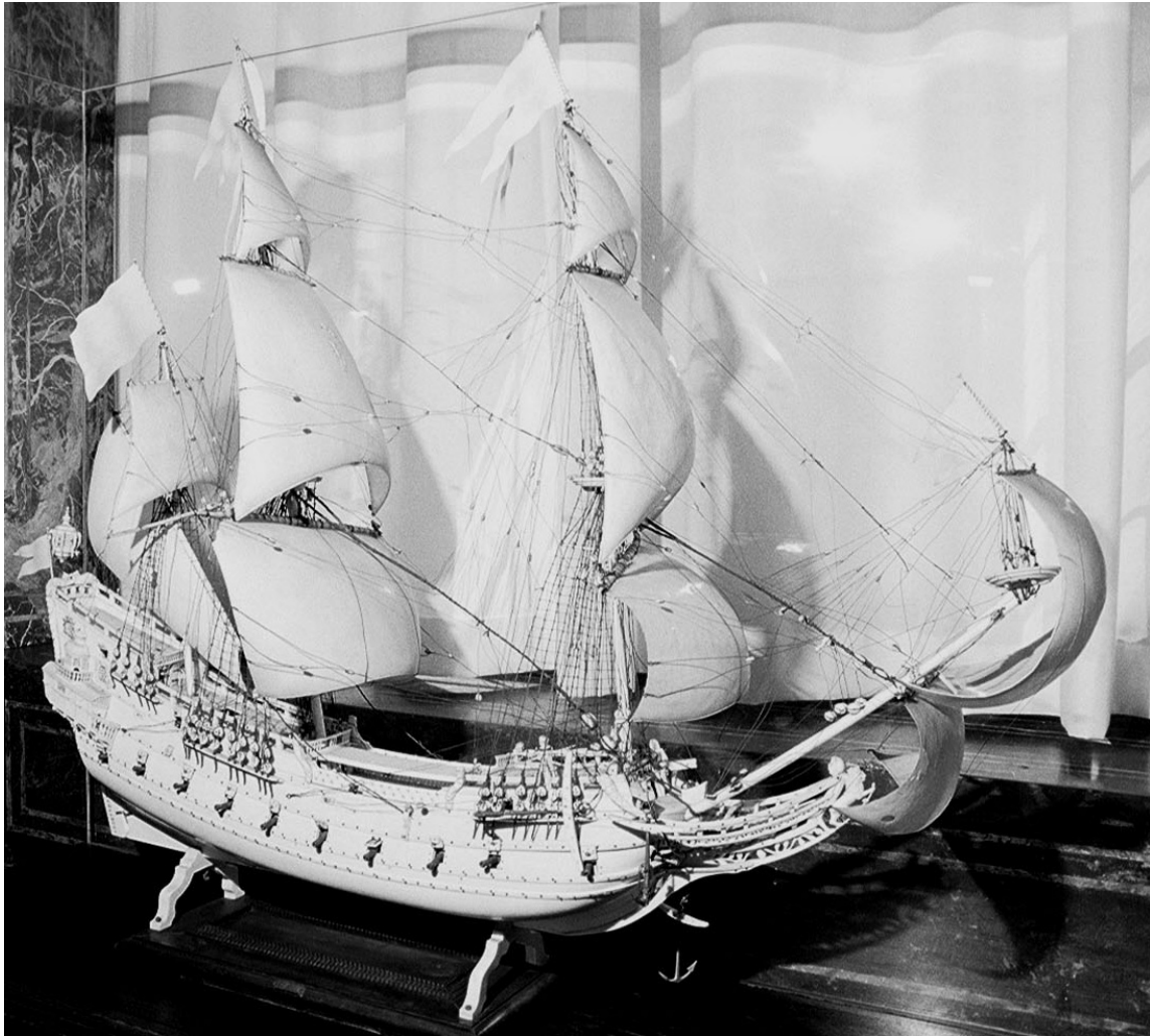
Fig. 51. The model of Norske Løve (1634) shows the extremely long bowsprit common to the early 17th century (in Rosenborg Castle, Copenhagen). (C. Corder)
