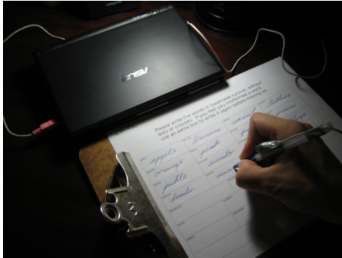
Fig. 10.: Pen Acoustic Emissions for Text and Gesture Recognition [41]
