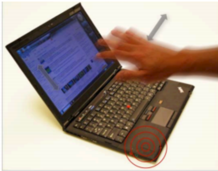
Fig. 11.: SoundWave uses the doppler effect to sense gestures [13]
