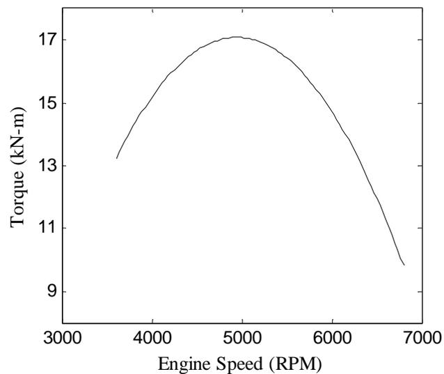
**Figure 14. Automobile engine torque curve used in demonstration.**
