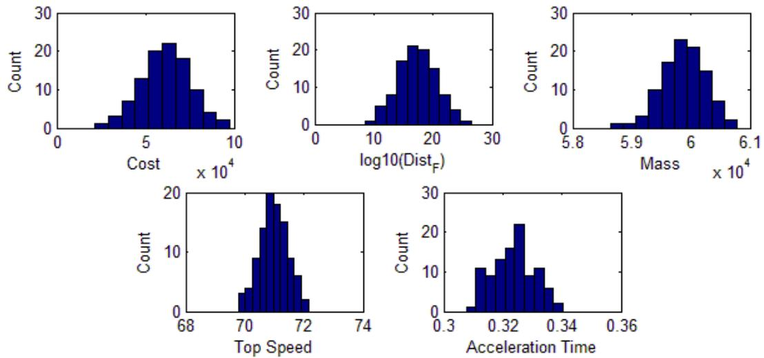
**Figure 19. Drivetrain cost, distance to failure, mass, top speed, and acceleration time histograms showing normal distributions.**
