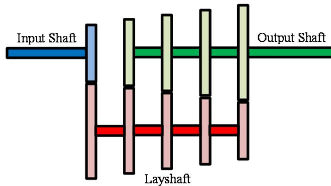
**Figure 15. Simple four-speed manual transmission physical configuration.**
