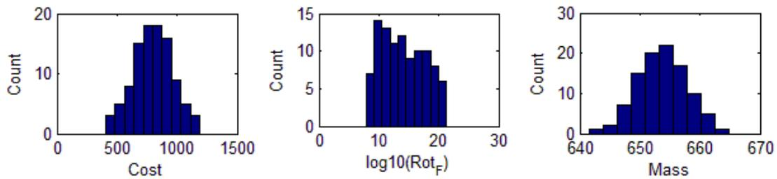
**Figure 18. Differential cost, rotations to failure, and mass attribute histograms showing normal distributions.**
