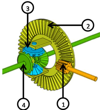
**Figure 16. Open differential physical configuration (1: input gear, 2: ring gear, 3: pinion gears, 4: side gears)**
