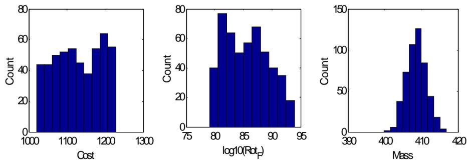
**Figure 21. Transmission cost, rotations to failure, and mass distribution histograms showing distributions.**
