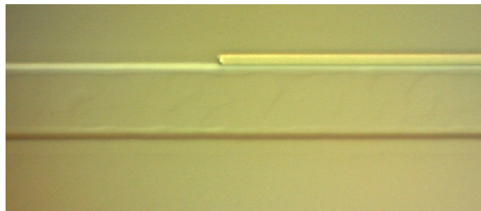
Fig. 50. Coupling region taper on fabricated sample.
