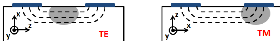
Fig. 21. Electrode orientation and substrate crystal cut for TE and TM polarization tuning with r_{33} .
