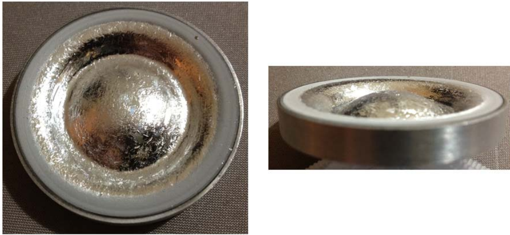
Fig. 40. Racetrack indentation on depleted metal target. Note that this is an Al target, but Ti targets show same behavior.
