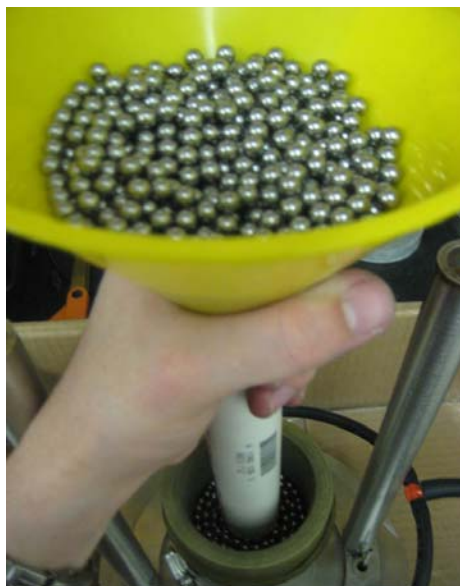
Figure 53: Material Slowly Being Deposited in the Mold.
