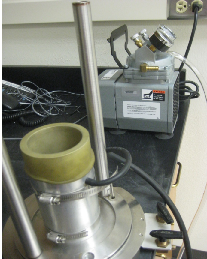
Figure 47: As can be Seen, the Split Mold is Held in Place with two Hoop Clamps. One at the Base of the Mold, One towards the Top. The Membrane is also in Place and Being Held Against the Sides of the Mold by the Vacuum Pump.
