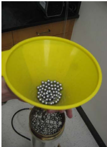
Figure 49: Material Flowing through the Mold while the Sieve Disperses the Material across the Area of the Tube.
