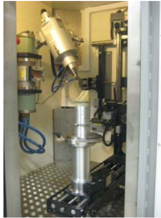
Figure 11: CT Scanner with Prepared Sample in Mold.
