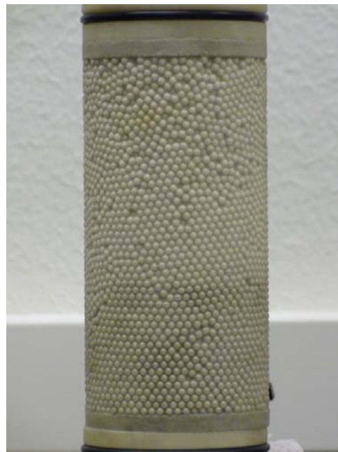
Figure 55: Final Sample Composed of 3 mm Spheres.
