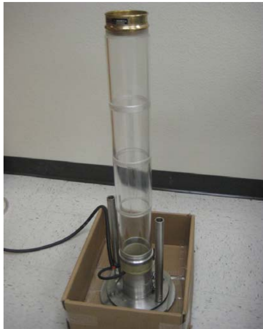
Figure 48: Mold and Triaxial Cell with Air Pluviation Tube in Place.
