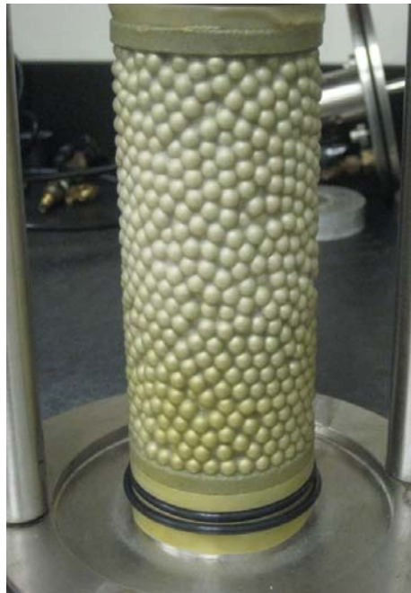
Figure 54: Final Sample Composed of 6 mm Spheres.
