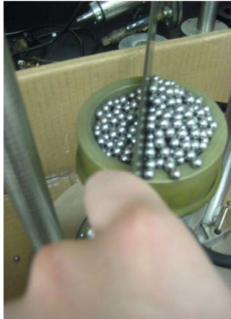
Figure 50: Removing Excess Material with a Steel Ruler.
