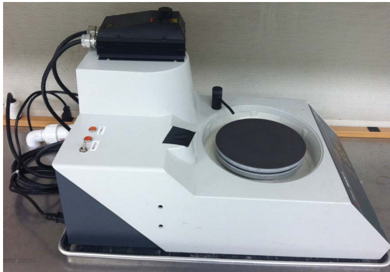
Fig. 27 Polishing setup consisting of polishing pad rotary, water spout, and speed controller.
