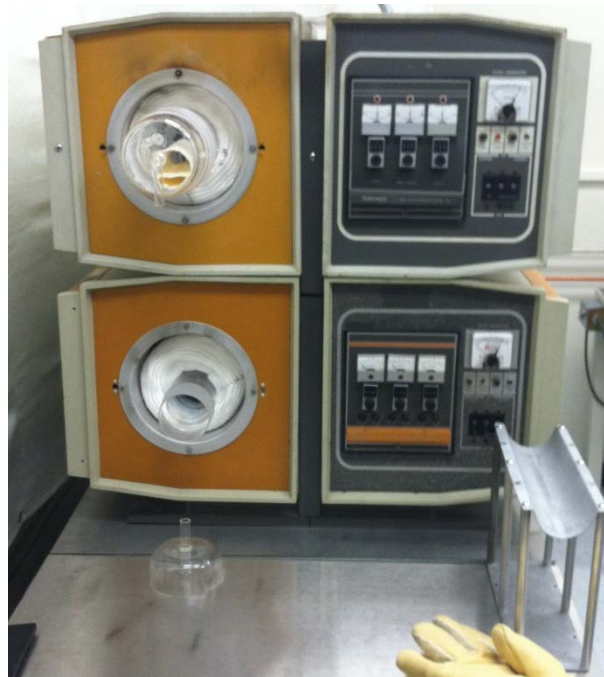
Fig. 26 Diffusion furnace used for the annealing of proton exchanged waveguides.
