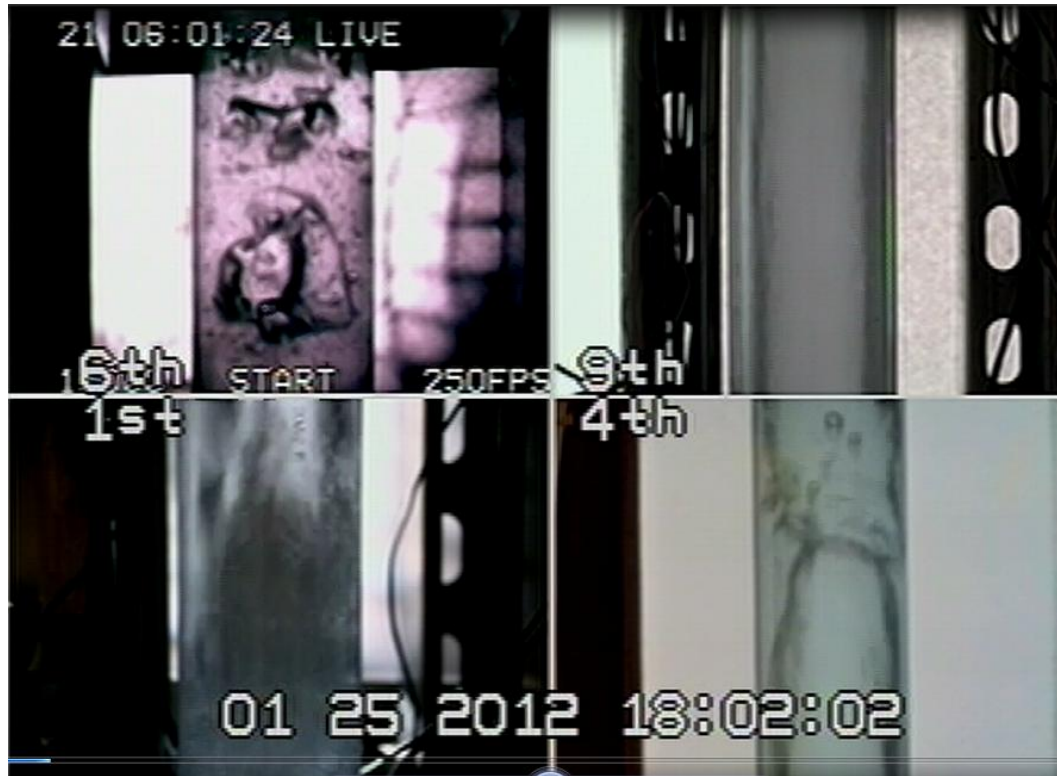
Figure 3.22 – Snapshot of a video captured during an experimental run. The videos are used to recognize the flow regime and analyze the axial development of the flow.
