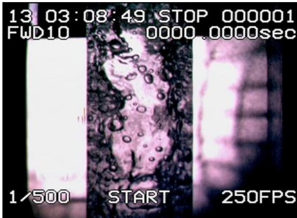
Figure 3.23 – Snapshot of a high-speed video captured during an experimental run. The high-speed videos are used to visualize fast change in the flow, which are difficult to capture with standard cameras.
