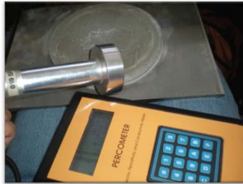
Figure 18: Determination of percometer penetration depth with cement paste cast on stainless steel at different thicknesses. The probe of the percometer uses a frequency of 40-50MHz.
