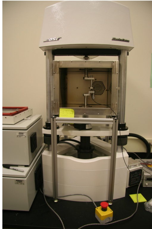
Figure 14: Bose ElectroForce 3200 testing machine used for uniaxial, sinusoidal loading for determination of damping in this research. Testing area is enclosed by a temperature chamber and also serves to isolate external vibrations.
