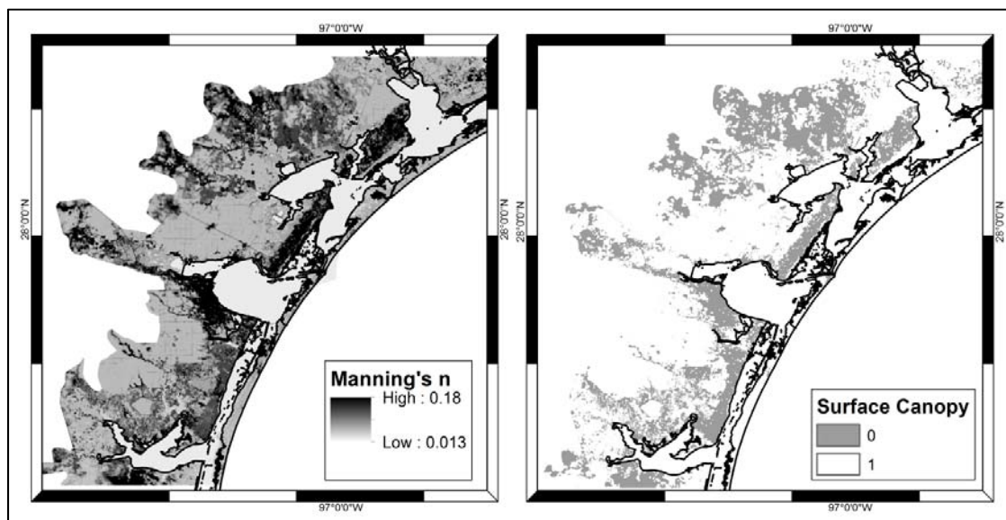
Figure 2.5: Geospatial representation of the frictional drag at the sea bottom by the Manning's n parameter (left) and the wind stress reduction through the surface canopy coefficient (right).
