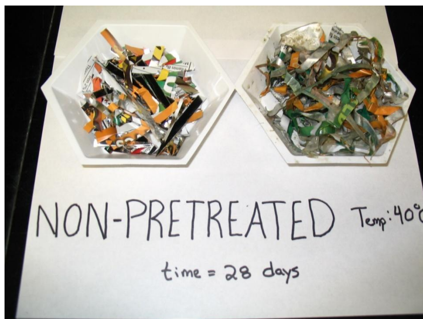
Figure 14-6. Picture comparing the pre- and post-reactor fermentation biomass for non-pretreated compostable bags at 40 °C after 28 days.
