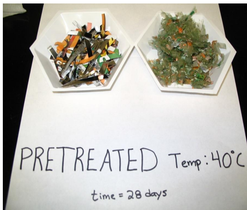
Figure 14-7. Picture comparing the pre- and post-reactor fermentation biomass for pretreated compostable bags at 40 °C after 28 days.
