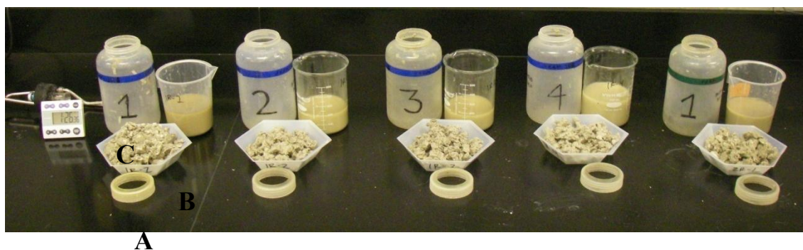
Figure 2-3. Photo of biomass during a 90-minute air exposure. A – filter solids in weigh boat; B – filter liquid in beaker; C – 1-L fermentation bottle
