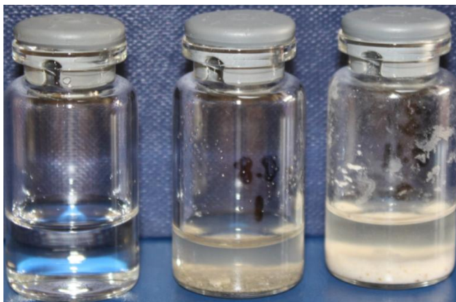
Figure 16-31. Glass sealed reaction vessels for glucose-utilization assay.
