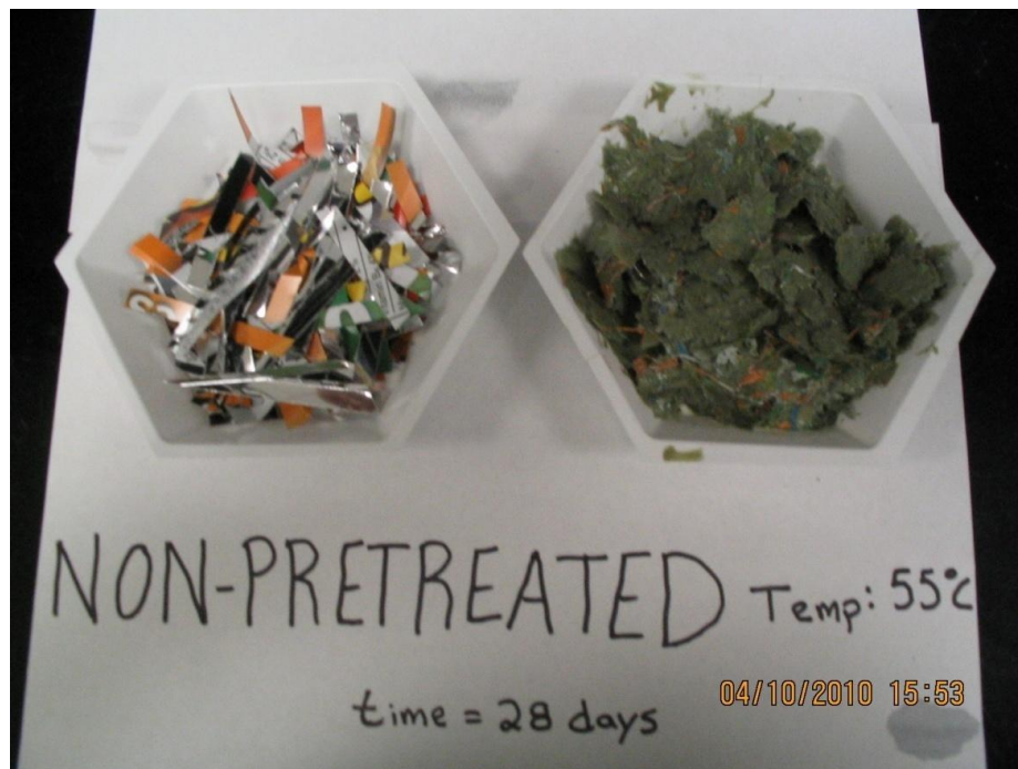
Figure 14-4. Picture comparing the pre- and post-reactor fermentation biomass for non-pretreated compostable bags at 55 °C after 28 days.
