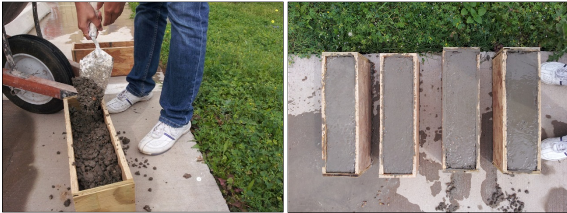
Figure 28. Beams during construction and after completion
