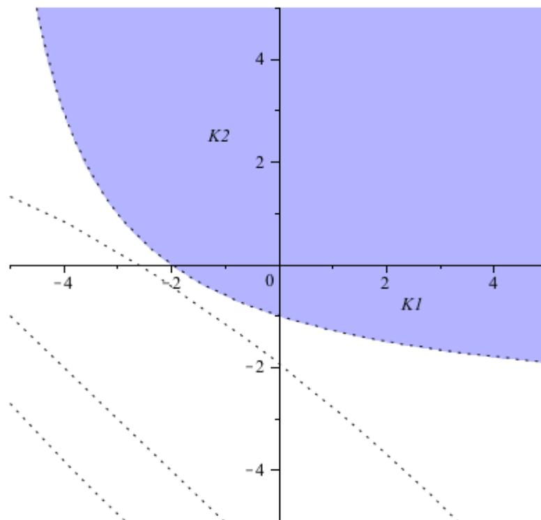
Fig.6. Theoretical Stabilizing Region (shaded area) for Example 2.
