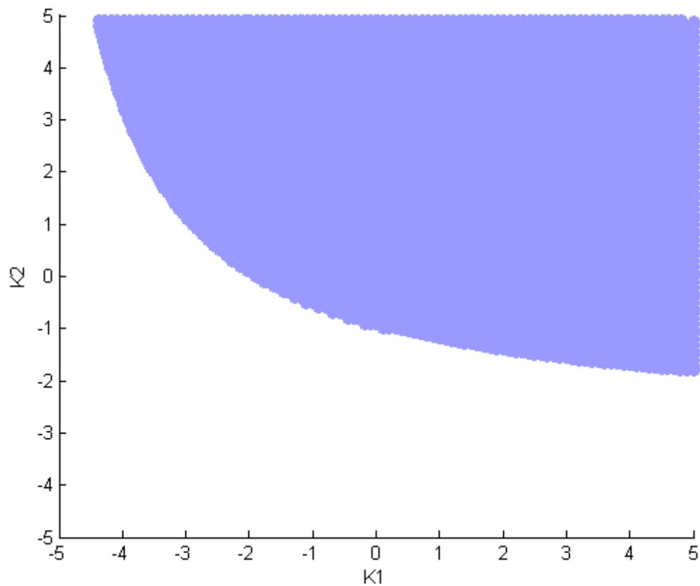
Fig.8. Stabilizing Region Using Proposed Approach for Example 2.
