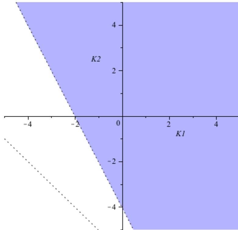
Fig.3. Theoretical Stabilizing Region (shaded area) for Example 1.
