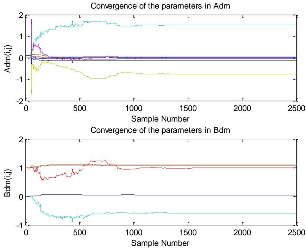
Fig.14. Convergence of Disturbance Model Parameters for  $\lambda = 0.9$ .
