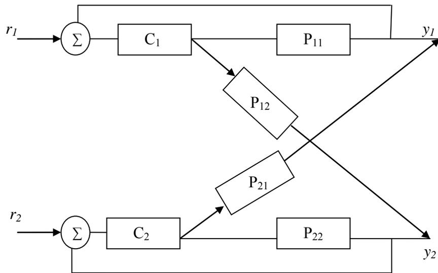
Fig.2. Internal Architecture of a TITO System.
