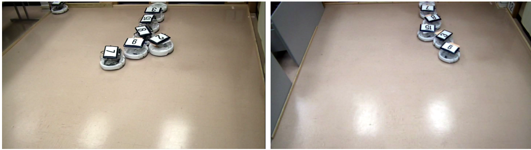
Fig. 11. A typical trial using 7 iRobot Create robots with \Delta q = 2 . A branch has been formed in the tree, but edges with robot #2 and robot #7 are not yet complete. Additional robots would need to perform EXTENDEGE operations for that to occur. This illustrates the asynchronous growth process involved in forming the RRT.
