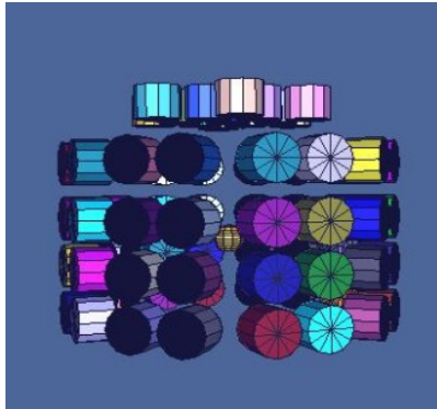
Fig. 4. Cylindrical Array of Liquid Scintillators Around Source.
