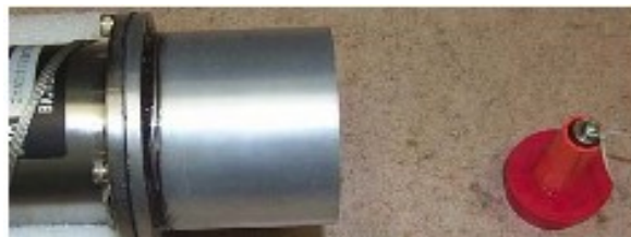
Fig. 2. A 2" x 2" BC501 Detector in Front of a ^{252}\text{Cf} Source. [10]
