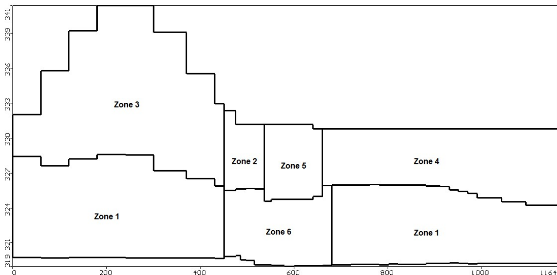
Figure 7. S_y is allocated into six zones. Zone 1 contains the lower layers except the Slough area. The upper layers are divided into 4 zones: the mound area, the area between the mound and riparian, the riparian and the area between the riparian and Canadian River
