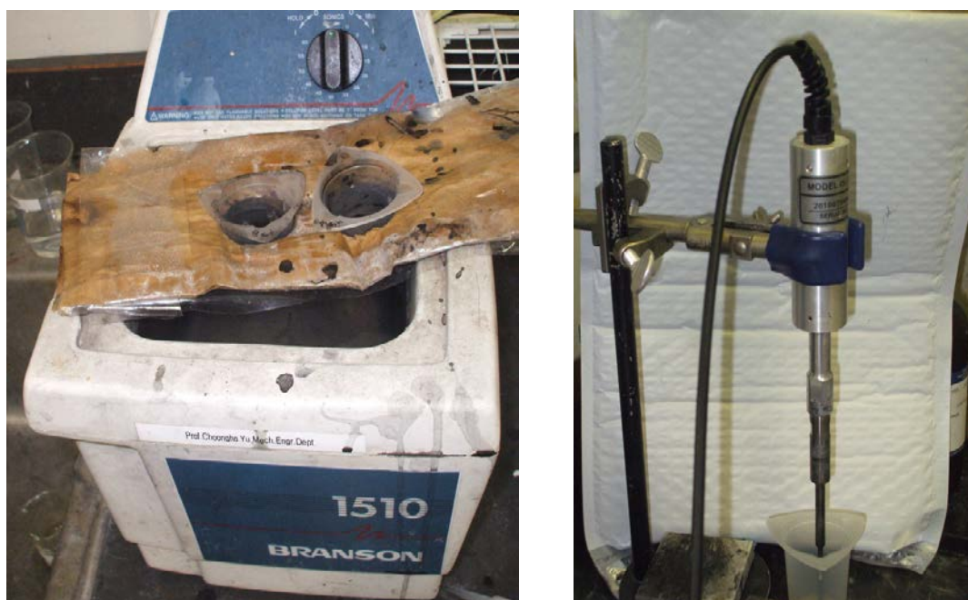
Figure 2. Bath type (left) and pen type (Right) sonicators used for dispersion.
