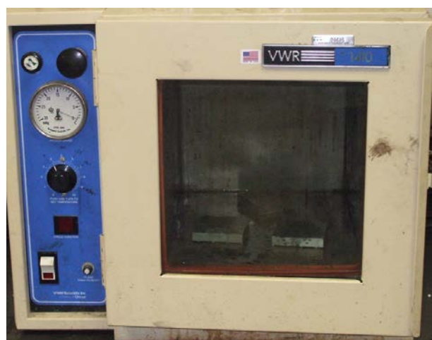
Figure 4. Drying was completed in a vacuum oven.
