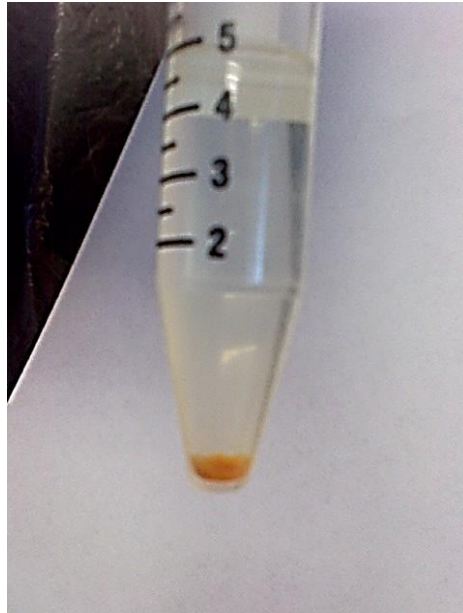
Fig. 64 —Sediments after coreflood with 2 wt% Zirconium lactate clay stabilizer.
