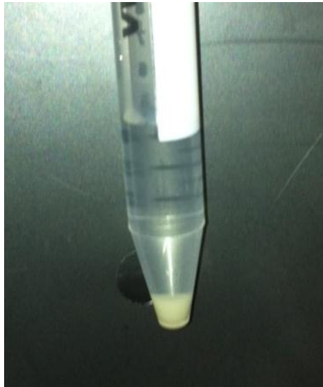
Fig. 45 —Sample 10, sediments are accumulated at the bottom at a flowrate of 2 cc/min.
