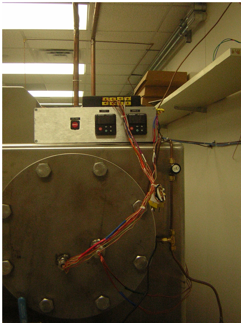
Fig. 3.13. Photograph of the CHTA data collection system outside of the glovebox.
