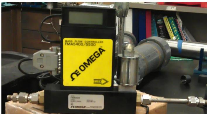
**Figure 3.8 OMEGA gas volume flowmeter**
