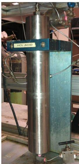
**Figure 3.2** Acid accumulator
