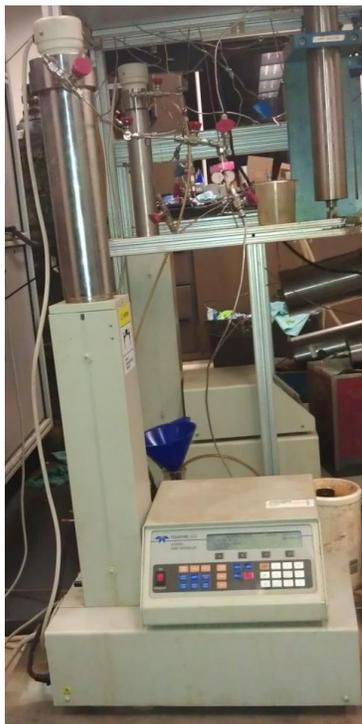
**Figure 3.1** Teledyne ISCO 500D syringe pump
