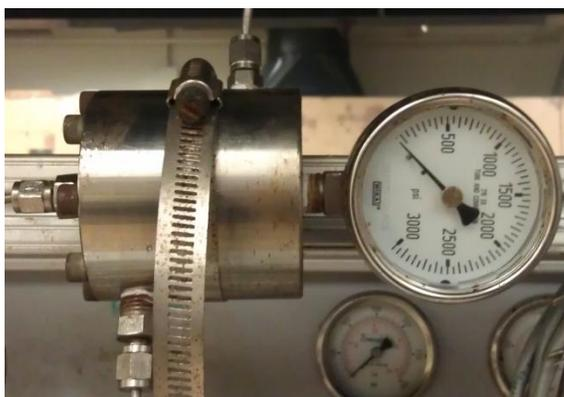
**Figure 3.6** Mity-Mite back pressure regulator
