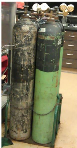
**Figure 3.9 Industrial grade-nitrogen cylinders**
