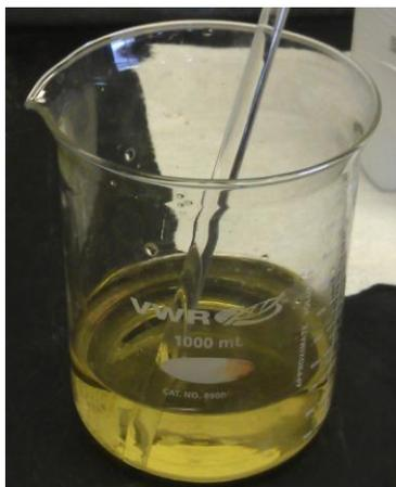
**Figure 3.19** A 15 wt% HCl solution with 2 wt% NaI added
