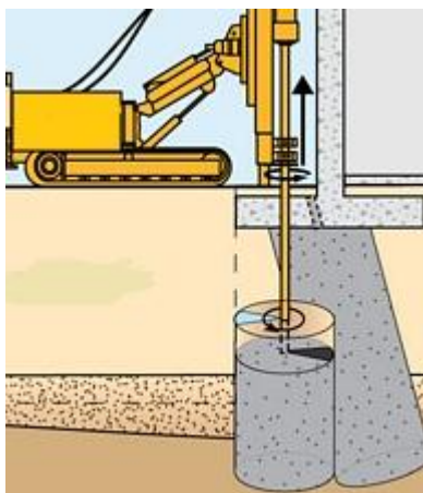
Figure 5- Schematic representation of the underpinning method used with jet-grouting (taken from [13])
