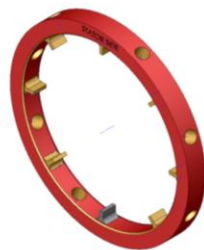
Figure 5. Isometric view of the swirl brake
