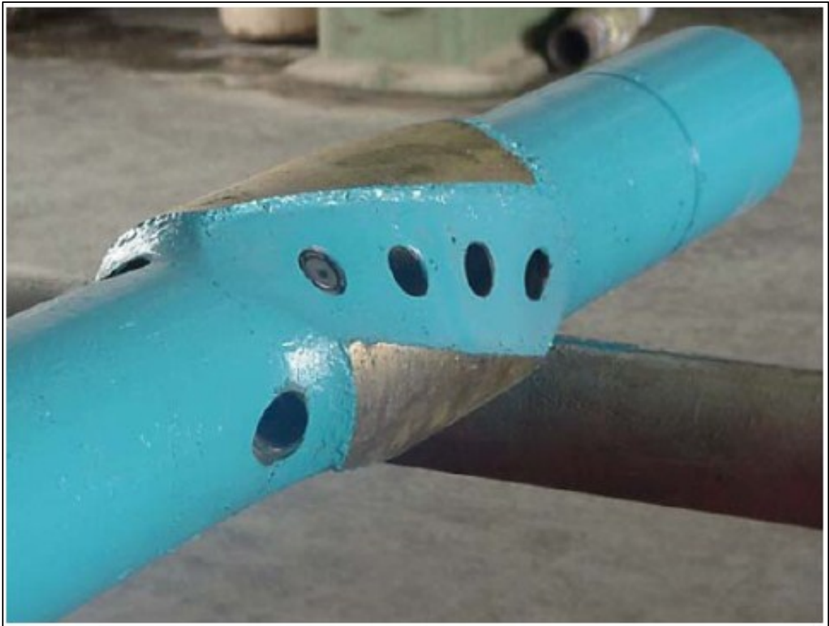
Fig. 1.2 – Acid jetting assembly (Ritchie et al. 2008)
