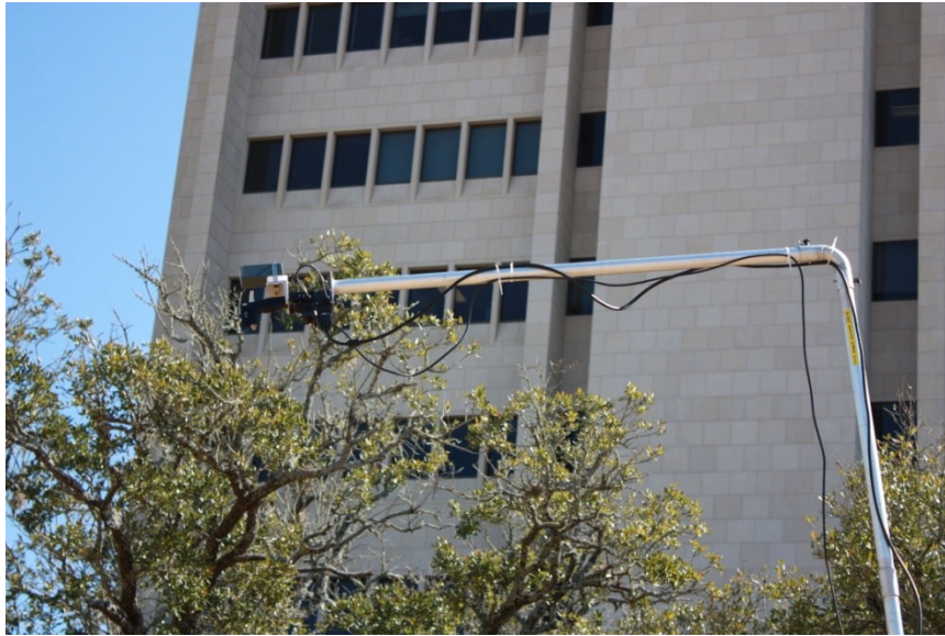
Fig. 14. The top part of the mast. The Pan-Tilt Unit, digital compass and ASD pistol are onboard there.
