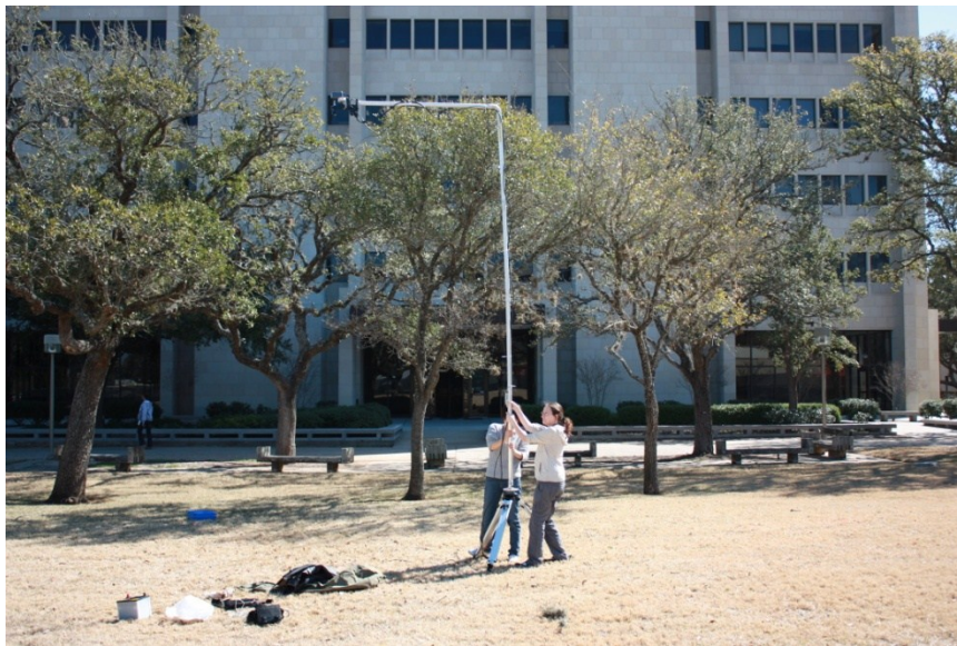
Fig. 13. The constructed multi-angle mast. This instrument can help to measure canopy BRDF.
