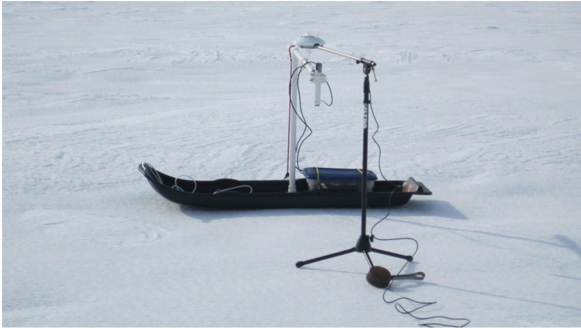
Fig. 6. EP16 and LI-COR instruments facing to each. The support structures were placed perpendicular to the sun with the instruments always pointing south of the mounting devices to minimize shadowing effects.
