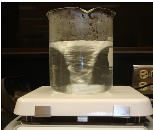
Fig. 11–Vortex formation with hot plate stirrer
