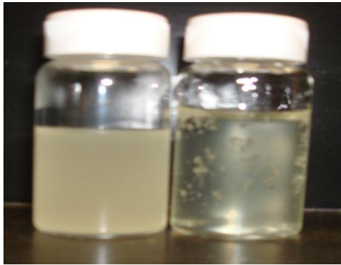
Fig. 22–(7000ppm/70000ppm) (HPAM/PEI) Samples showing difference in pH.
