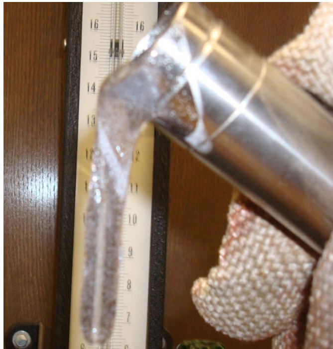
Fig. 29 - HPAM/CrAc gel (7000ppm/500ppm) sudden gelation @212°F
