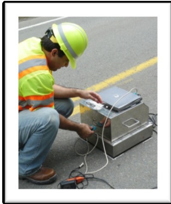
FIGURE 7 A technician setting up the CT Meter in the field.
