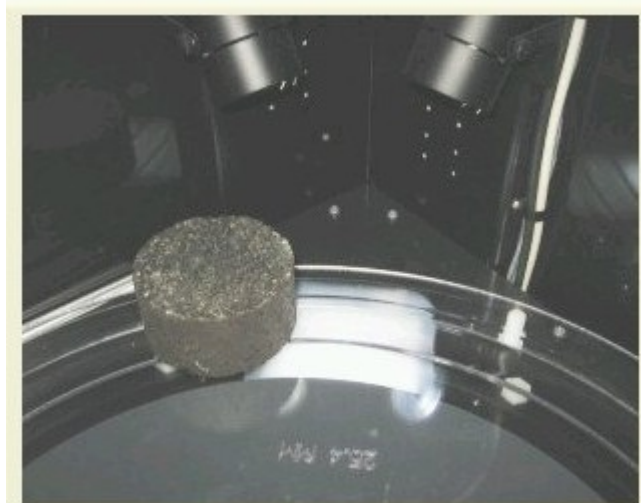
FIGURE 21 Pavement core during scanning in AIMS.
