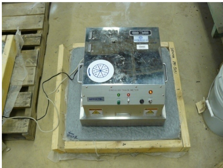
FIGURE 17 Fabricated concrete slab with rough surface texture being measured by the CT Meter. The diagram of the circumferential segments into which the data are divided can be seen on the top of the CT Meter.
