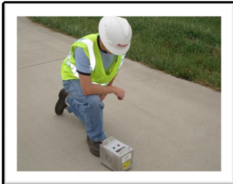
FIGURE 10 Technician using the Ames laser texture scanner to measure pavement macrotexture (46).
