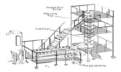
Figure 2.4 Schematic of facility used in modeling [21]
