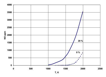
Figure 2.1 Thermal NO<sub>X</sub> equilibrium calculations for methane at different excess air
