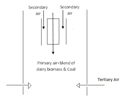
Figure 4.4 LNB model schematic
