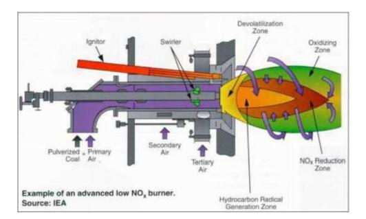
Figure 2.2 LNB example (adapted from [16])
