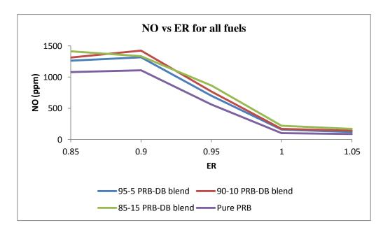
Figure 5.9 Comparison of NO emissions for blended to unblended fuel
