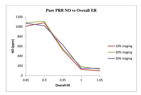
Figure 5.2 Pure PRB NO vs. overall ER
