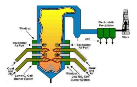
Figure 1.1 Schematics of a coal burner
