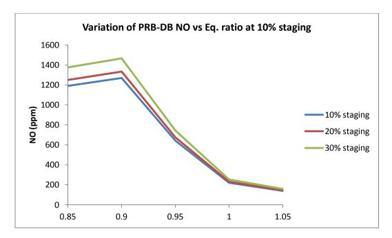
Figure 5.7 PRB vs. ER for different staging percentages
