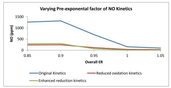
Figure 5.11 Parametric evaluation of pre-exponential factors on NO
