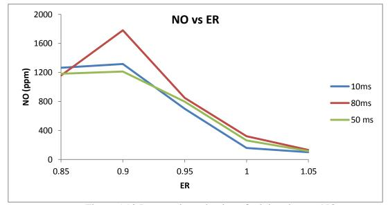
Figure 5.10 Parametric evaluation of mixing time on NO
