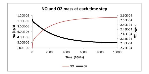
Figure 5.5 NO and O<sub>2</sub> concentration along the burner for pure PRB at ER=0.95 and 10% staging
