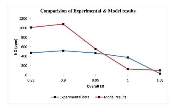
Figure 5.4 Comparison of experimental and model results for pure PRB & 10% staging
