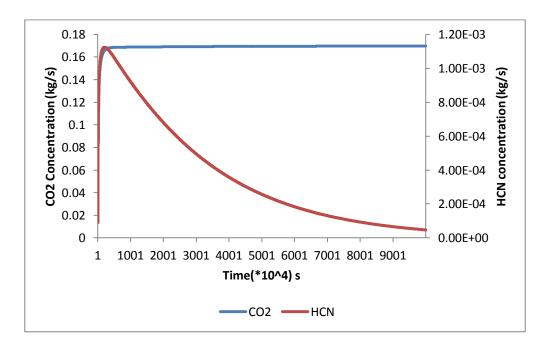
Figure 5.6 CO<sub>2</sub> and HCN concentration for pure PRB 10% staging ER=0.85
