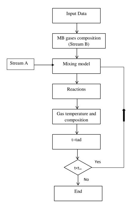
Figure 5.1 Numerical model algorithm
