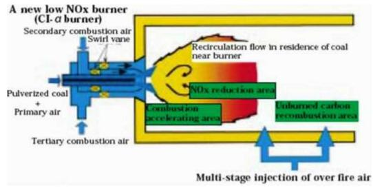
Figure 2.3 NOx reduction area in LNB (adapted from [18])
