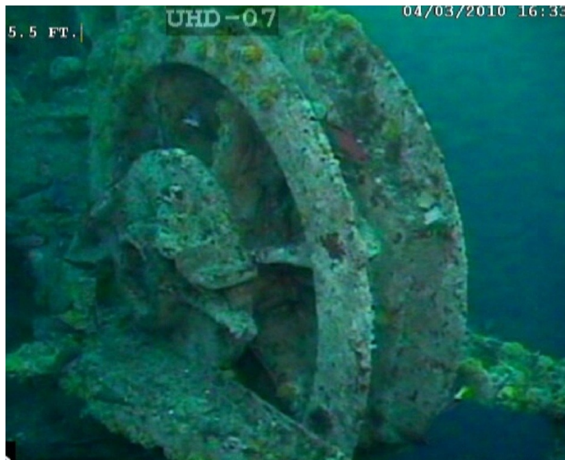
Figure 5: Fairlead Marine Growth After Service Time in the Gulf of Mexico
