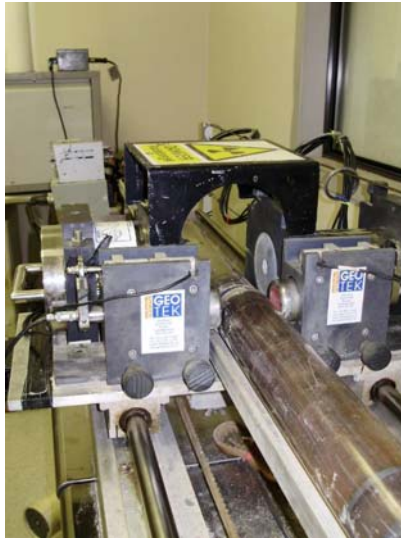
Fig. 5.5. Photograph of multi-sensor core logger.
