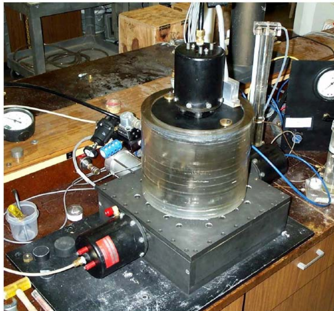
Fig. 2.12. Photograph of the University of California, Berkeley bidirectional cyclic simple shear device (After Kammerer et al., 1999).
