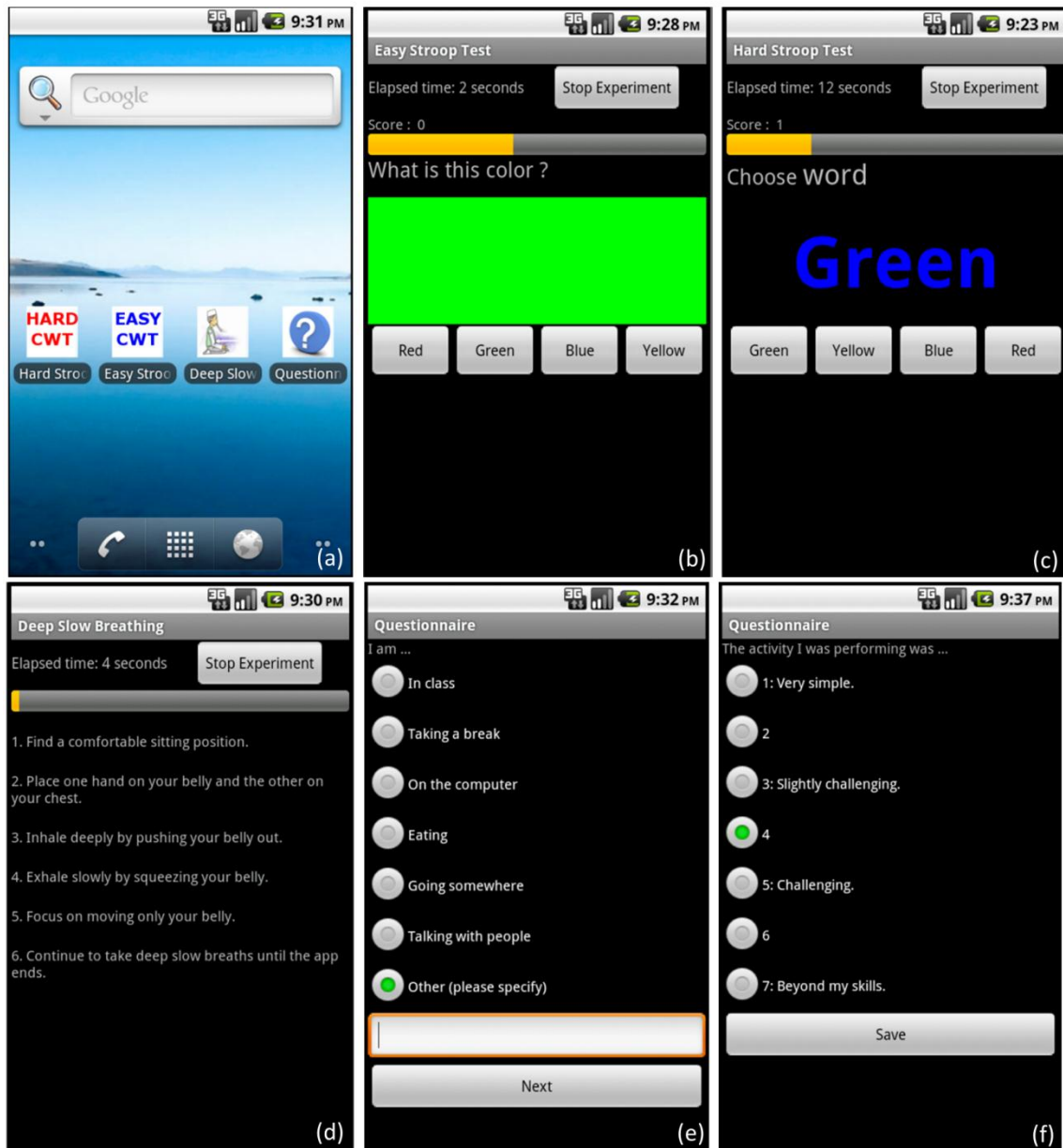
Figure 55. Screenshots of the ambulatory stress monitoring software in Android platform. (a) Android main screen for the four apps, (b) easy Stroop color word test, (c) hard Stroop color word test, (d) spontaneous deep breathing task, (e) questionnaires for the subject's context, and (f) questionnaires for the subject's stress level.
