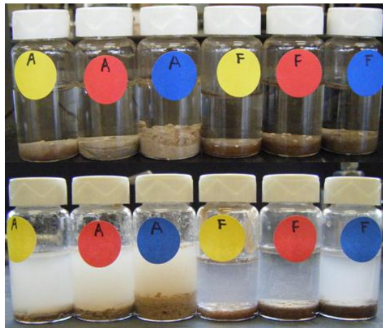
Fig. 17—We soaked and shook the samples in synthetic seawater for one hour before pull-out tests. The upper one is shown what samples look like before shaking. The lower one tells barite in A epoxy system is easier to come out after shaking.
