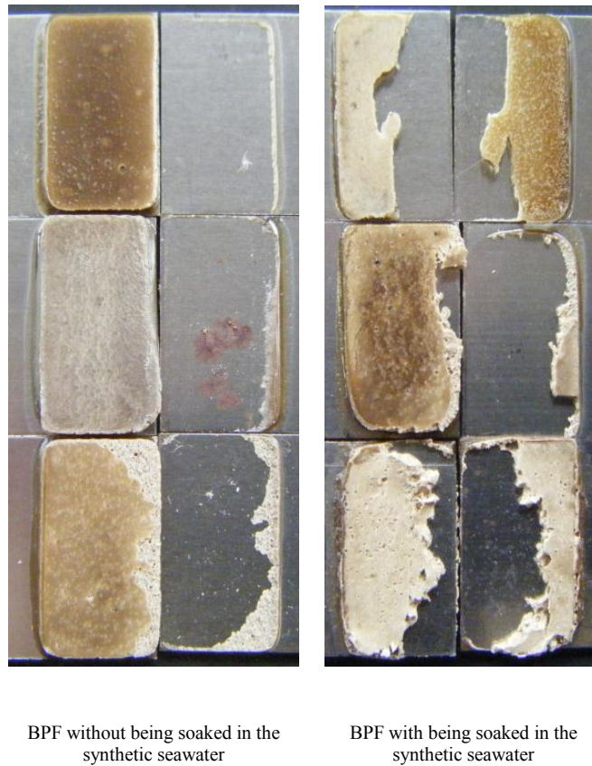
Fig. 22– After shear bond strength at 200 °F, for BPF system, the texture on the right look looser and the contact area seems less than the ones on the left.
