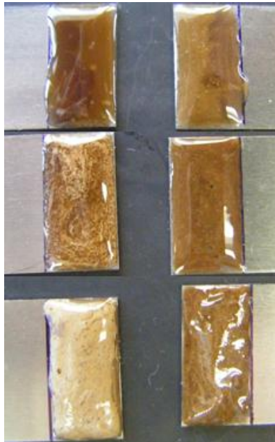
Fig. 18 —After one hours of being soaked in synthetic seawater, the epoxy was mixed with synthetic seawater. The left three samples are for A epoxy system. The right three are F epoxy system's samples
