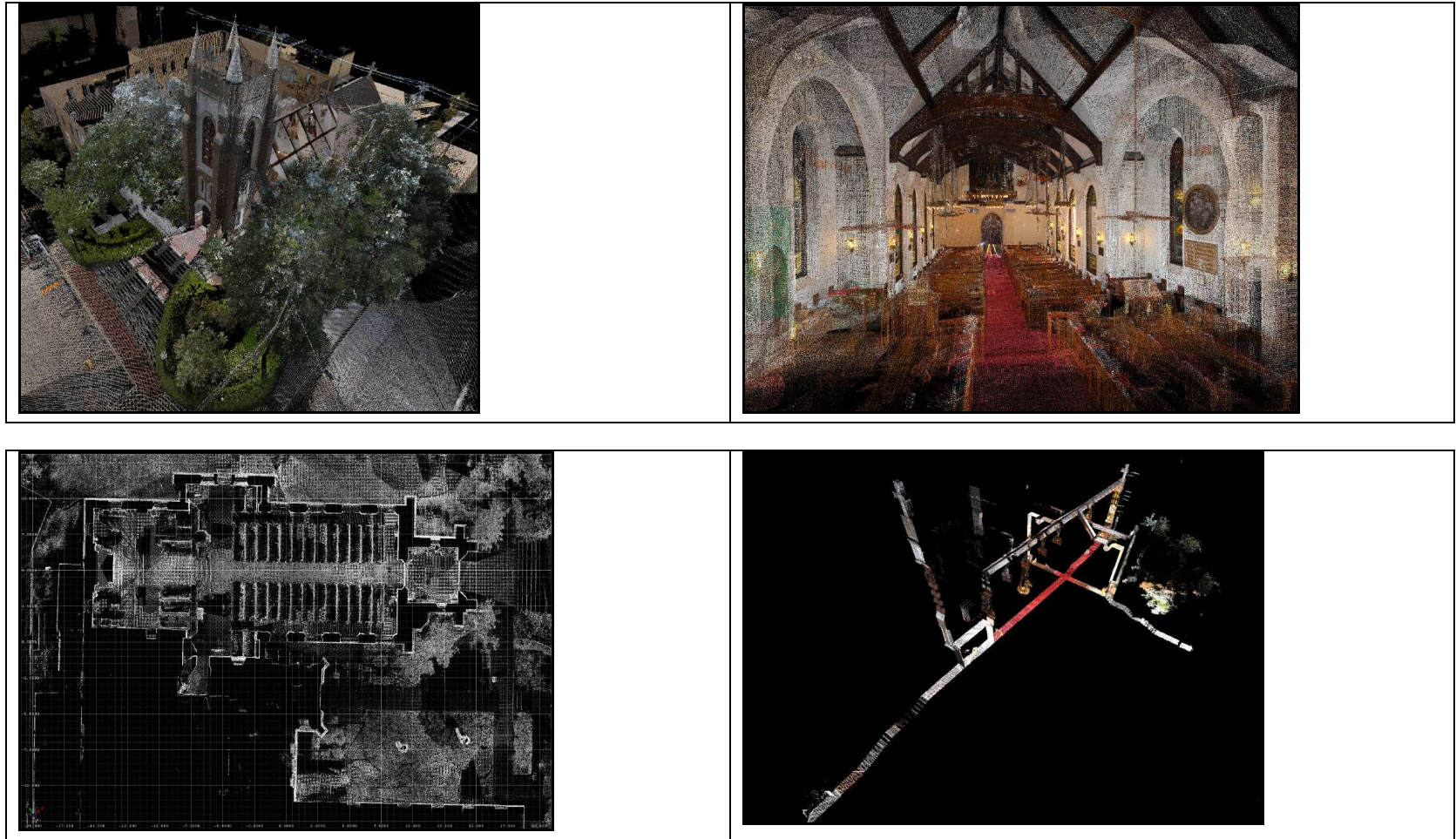
Fig. 15. The above left image demonstrates the overall look of the structure in 3-D point-cloud. The above right image shows the interior space. As the image demonstrates, scanned data consists of millions of data points. The below left image is a good example of how point-cloud can be sliced to produce plan representation. The image shows the planimetric cut. The below right image shows the section slices to determine the vertical measurements of the cross-sections. (Copyright: Center for Heritage Conservation.)
