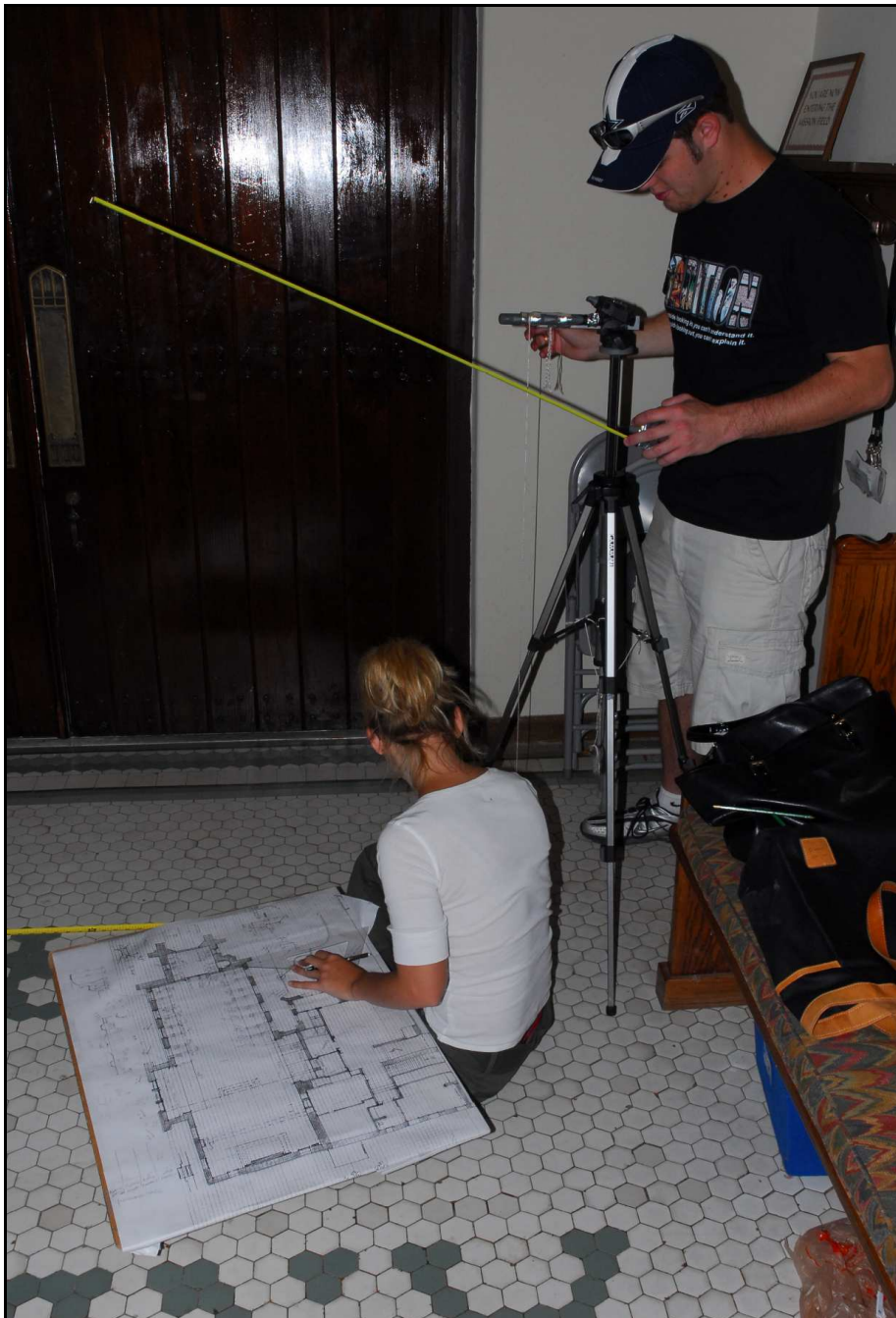
Fig. 10. The CHC team worked at the St. Andrews Episcopal Church during the documentation campaign in 2008. The team members gathered horizontal measurements to produce the plan drawing. (Copyright: Center for Heritage Conservation.)
