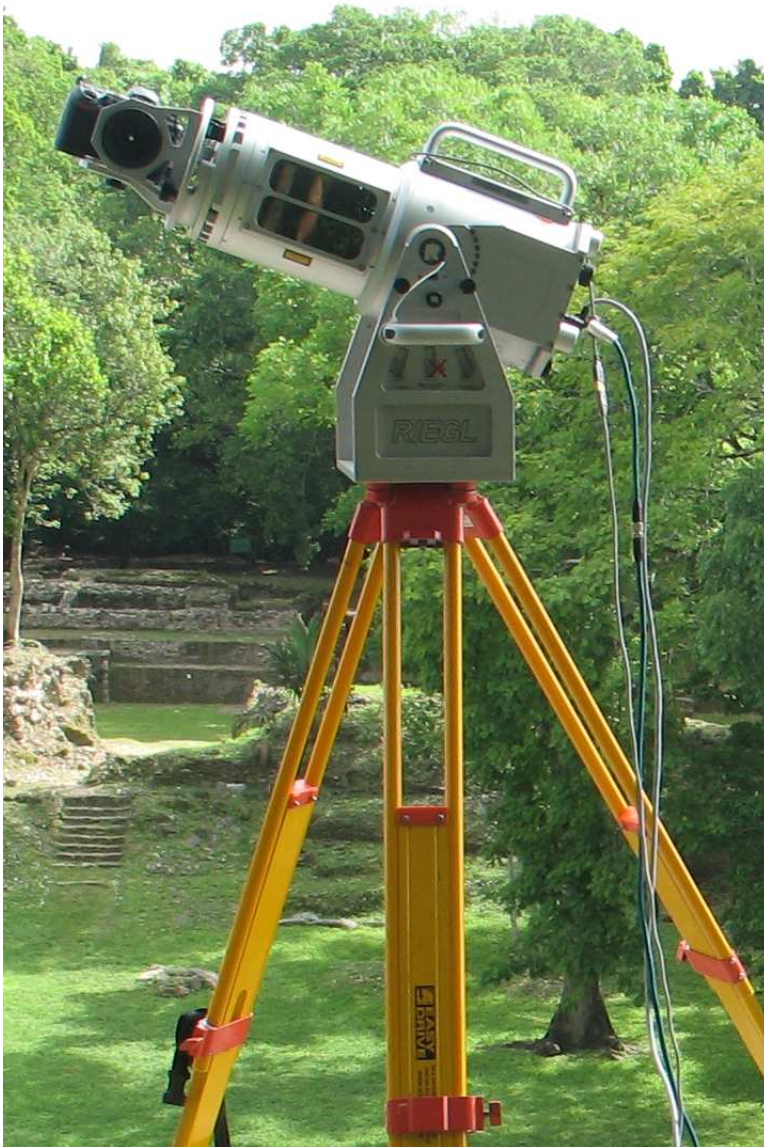
Fig. 14. The CHC documentation team used this 3-D laser scanner during the documentation of St. Andrews Episcopal Church in Bryan, Texas in 2008. (Copyright: Center for Heritage Conservation)
